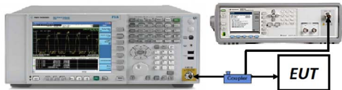
Figure 7-4. Test Instrument & Measurement Setup
