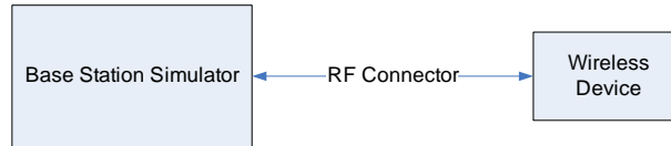
Figure 8-2 Power Measurement Setup
