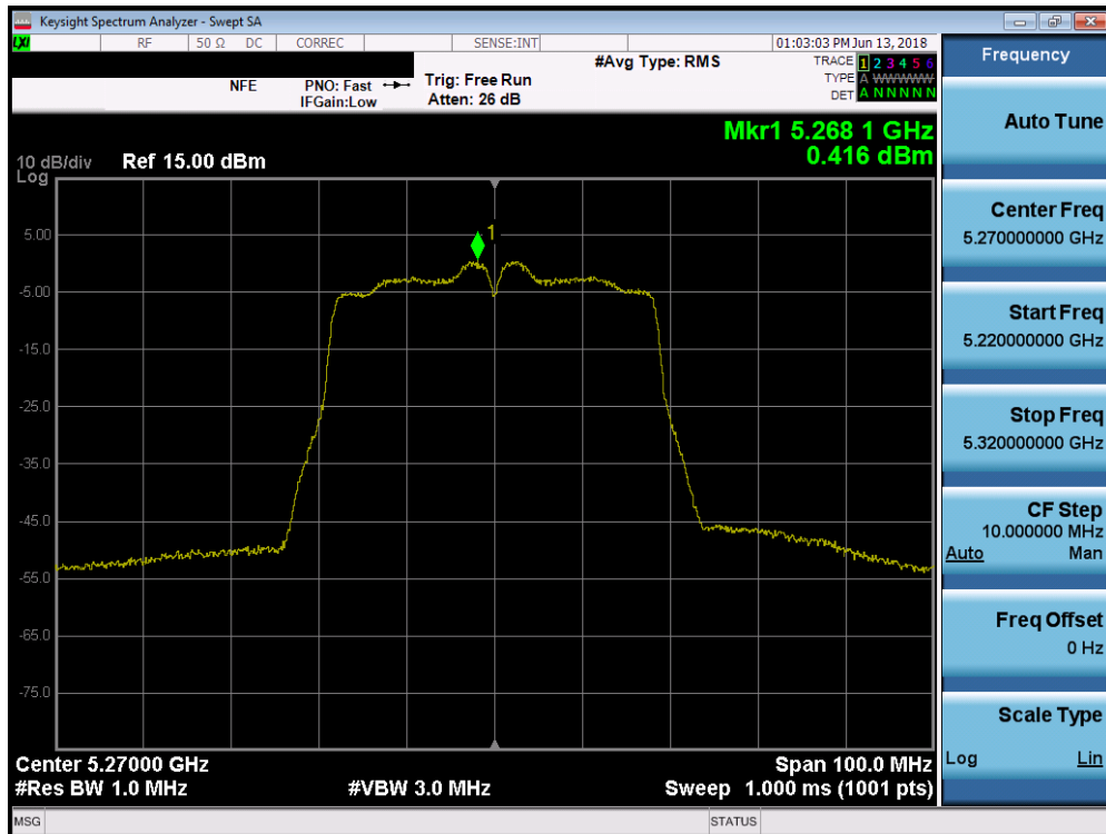
Plot 7-94. Power Spectral Density Plot (40MHz BW 802.11n (UNII Band 2A) – Ch. 54)
