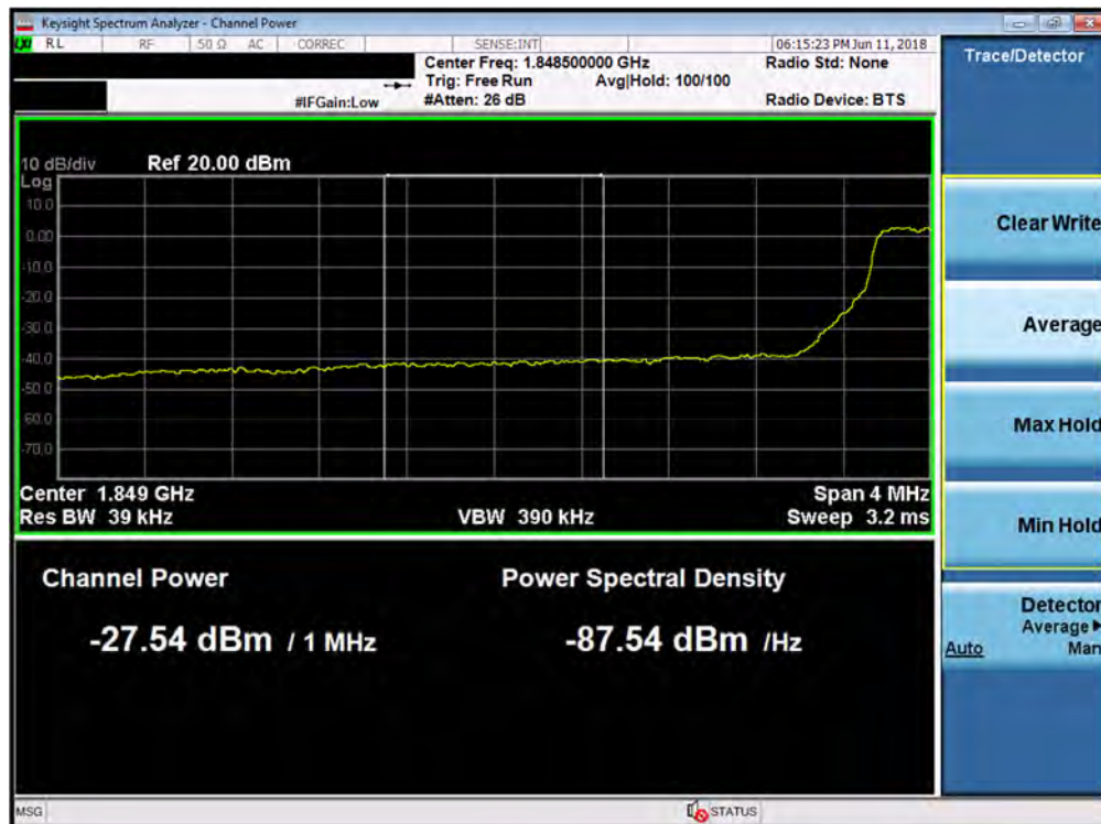
Plot 7-229. Lower Extended Band Edge Plot (Band 2 - 5.0MHz QPSK - Full RB Configuration)
