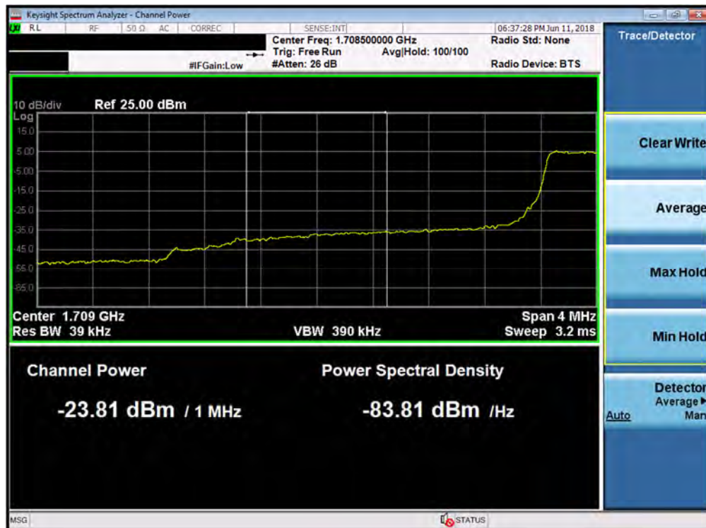
Plot 7-197. Lower Extended Band Edge Plot (Band 4 - 3.0MHz QPSK - Full RB Configuration)
