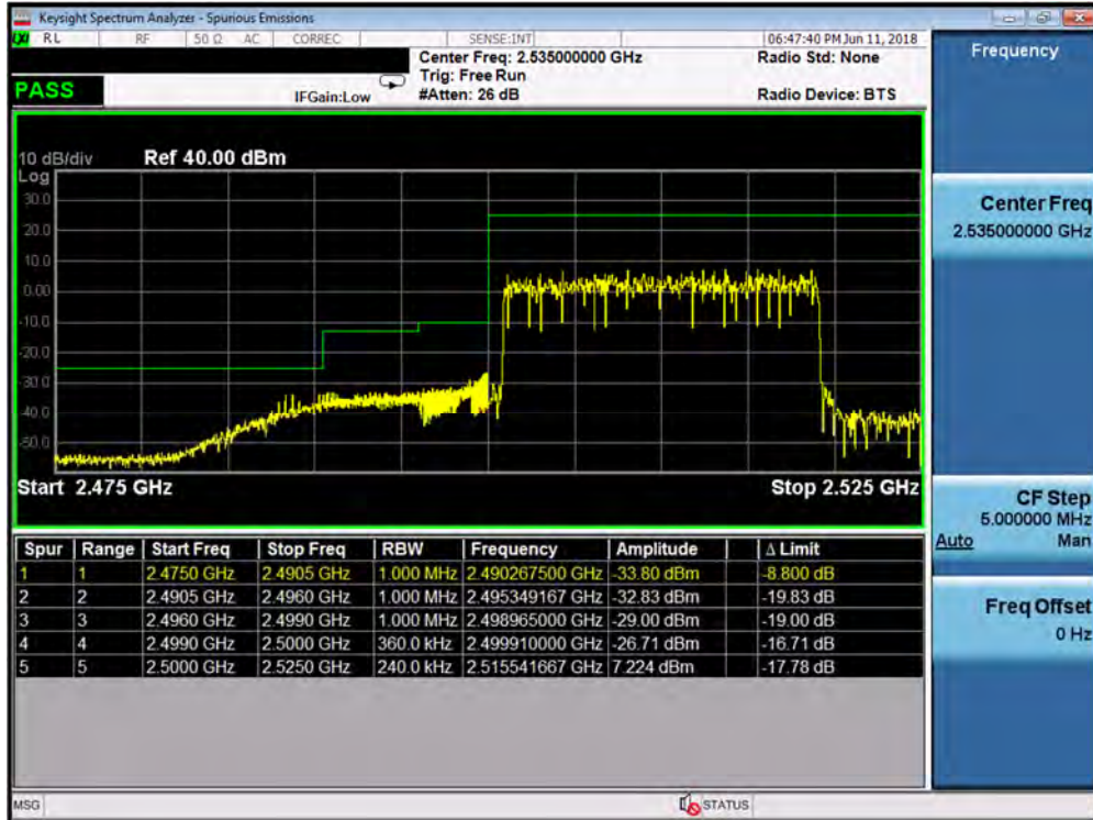
Plot 7-258. Lower Band Edge Plot (Band 7 - 20.0MHz QPSK - Full RB Configuration)
