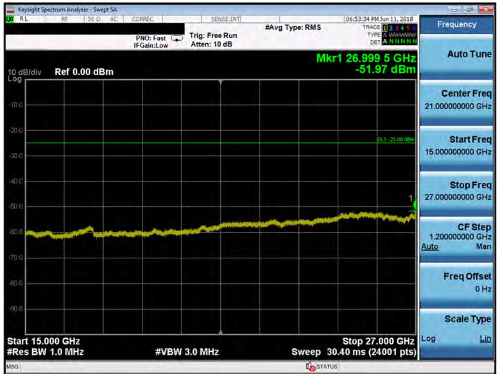
Plot 7-156. Conducted Spurious Plot (Band 7 - 5.0MHz QPSK - RB Size 1, RB Offset 0 - High Channel)
