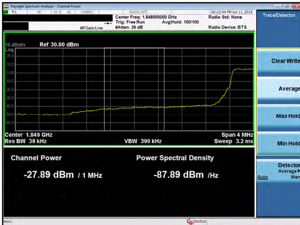
Plot 7-223. Lower Extended Band Edge Plot (Band 2 - 3.0MHz QPSK - Full RB Configuration)
