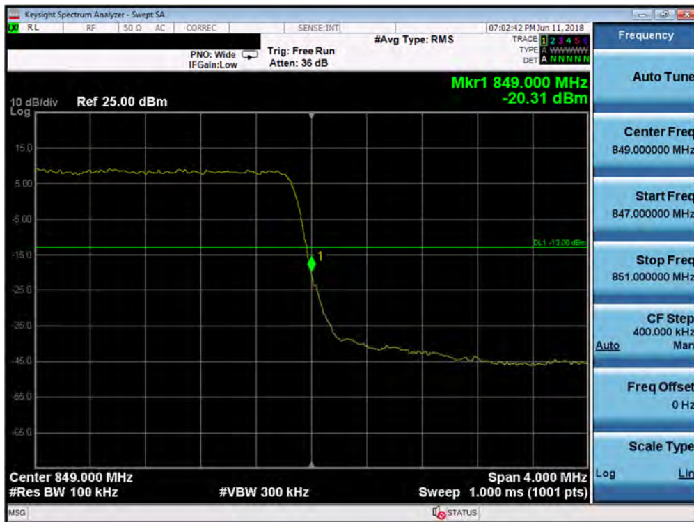
Plot 7-185. Upper Band Edge Plot (Band 26/5 - 3.0MHz QPSK - Full RB Configuration)
