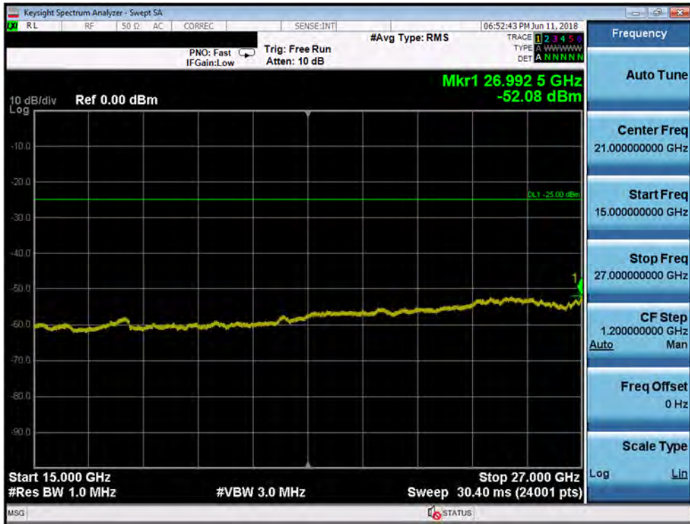
Plot 7-150. Conducted Spurious Plot (Band 7 - 5.0MHz QPSK - RB Size 1, RB Offset 0 - Low Channel)
