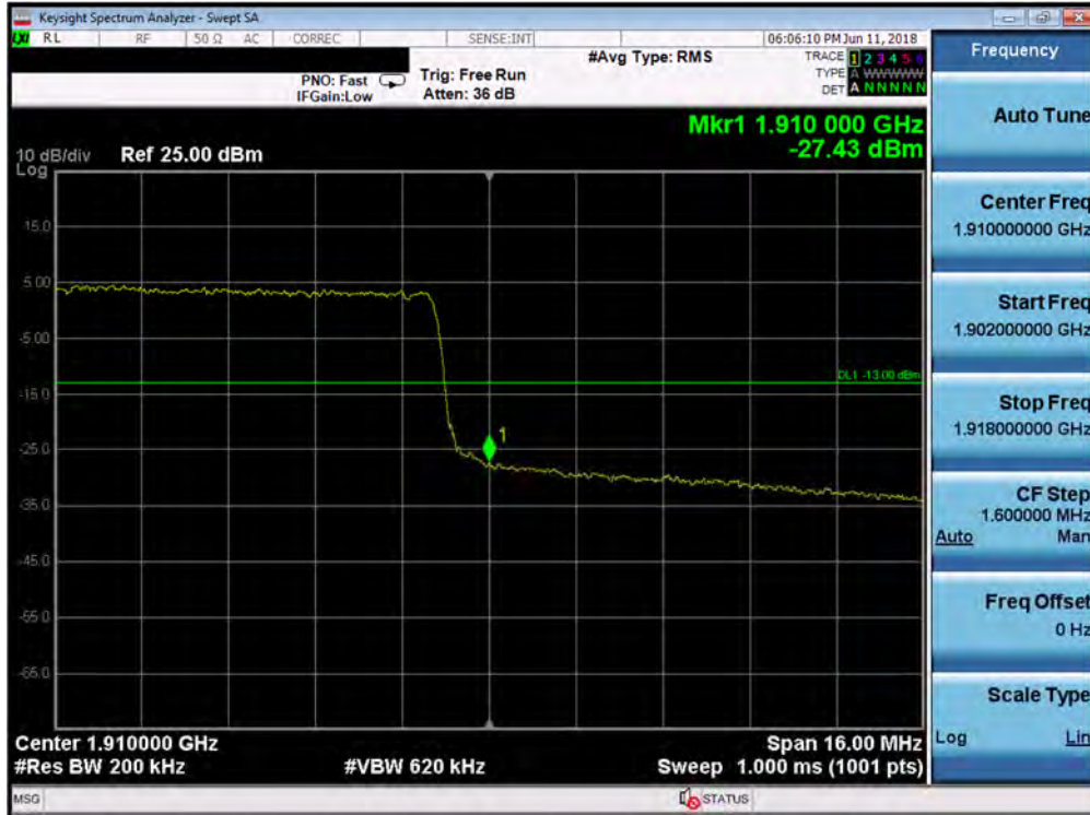
Plot 7-248. Upper Band Edge Plot (Band 2 - 20.0MHz QPSK - Full RB Configuration)
