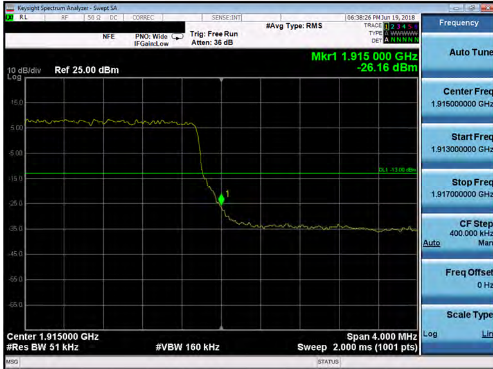
Plot 7-232. Upper Band Edge Plot (Band 25 - 5.0MHz QPSK - Full RB Configuration)
