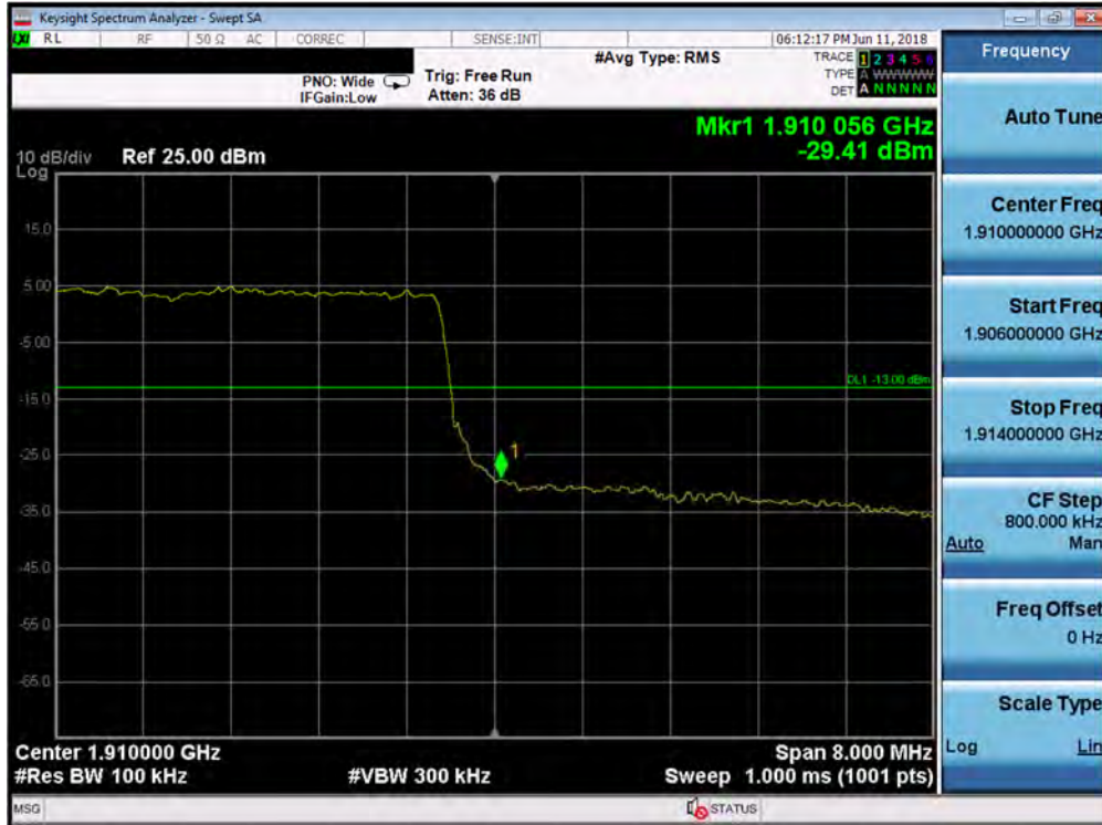
Plot 7-236. Upper Band Edge Plot (Band 2 - 10.0MHz QPSK - Full RB Configuration)
