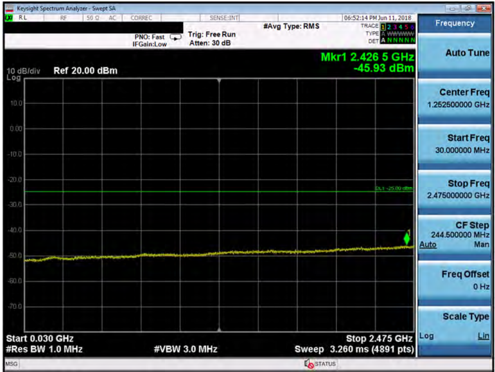
Plot 7-148. Conducted Spurious Plot (Band 7 - 5.0MHz QPSK - RB Size 1, RB Offset 0 - Low Channel)
