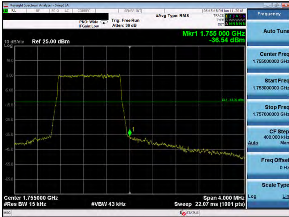
Plot 7-194. Upper Band Edge Plot (Band 4 - 1.4MHz QPSK - Full RB Configuration)
