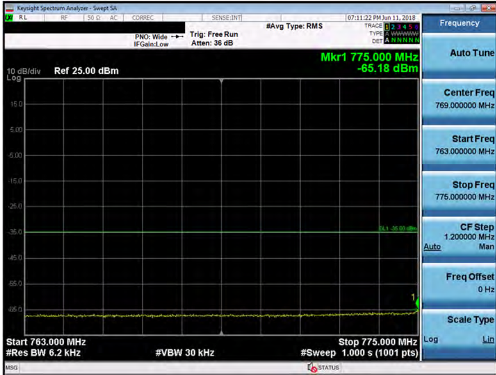
Plot 7-178. Lower Emission Mask Edge Plot (Band 13 – 10.0MHz QPSK – Full RB Configuration)
