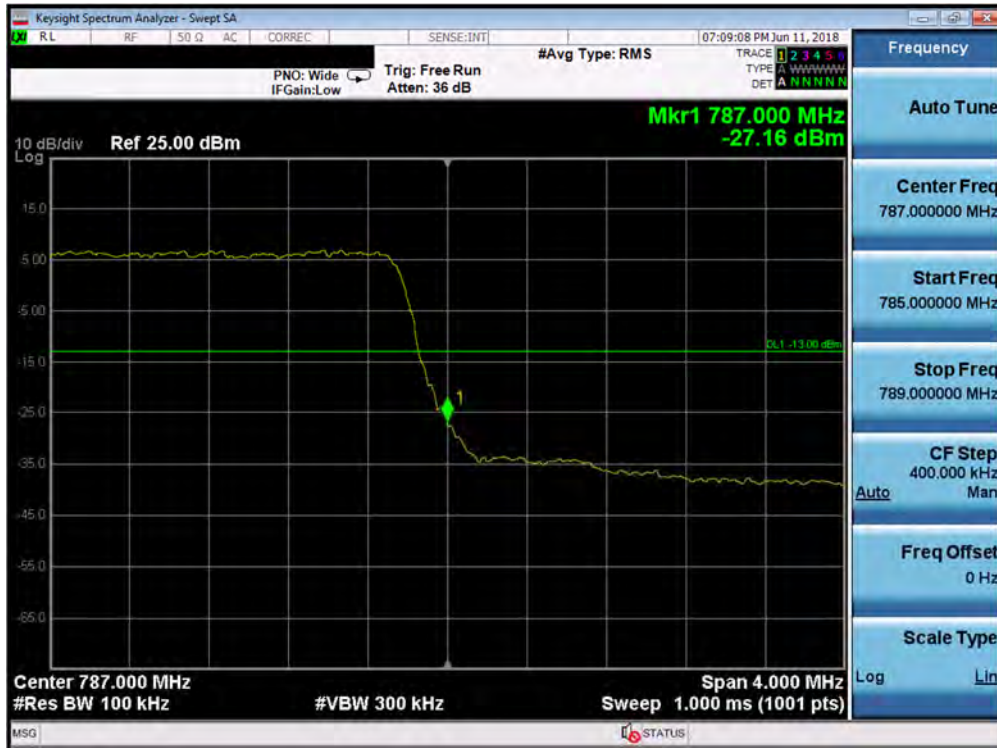
Plot 7-176. Upper Band Edge Plot (Band 13 - 5.0MHz QPSK - Full RB Configuration)
