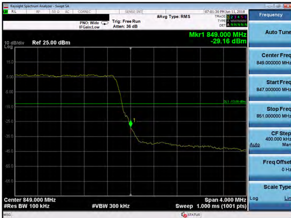
Plot 7-187. Upper Band Edge Plot (Band 26/5 - 5.0MHz QPSK - Full RB Configuration)
