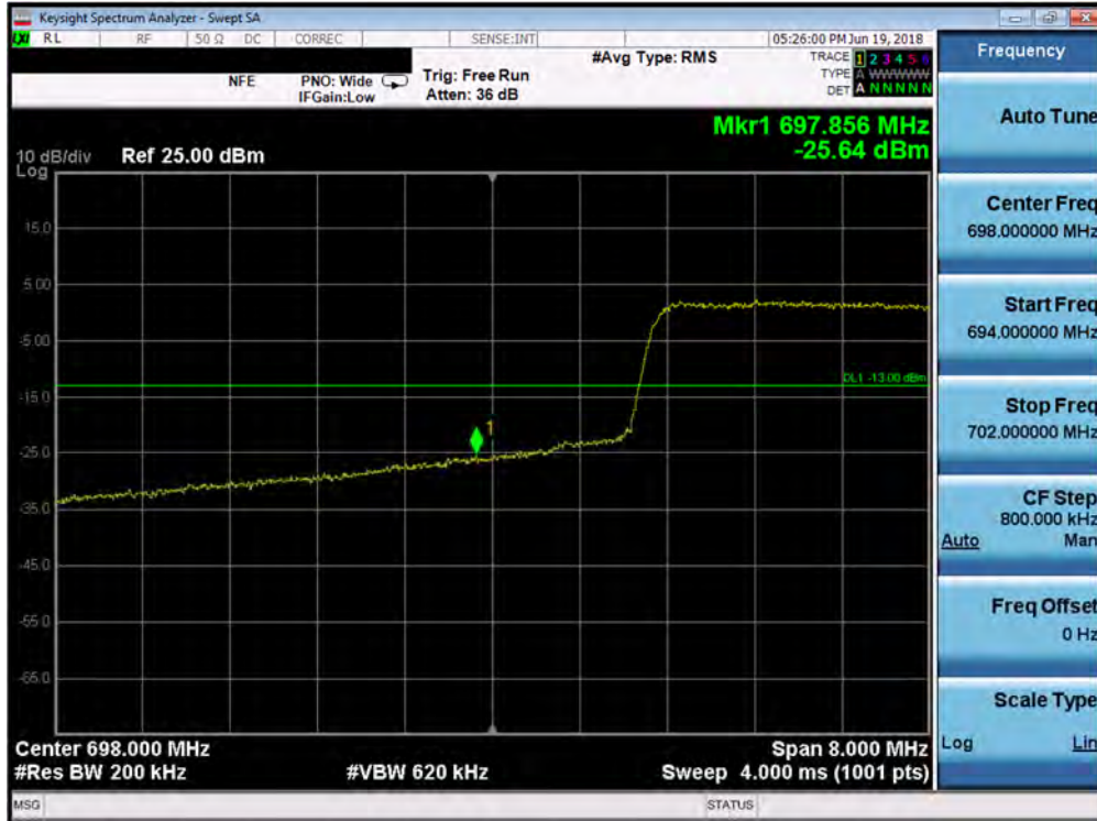
Plot 7-172. Lower Band Edge Plot (Band 12 - 10.0MHz QPSK - Full RB Configuration)
