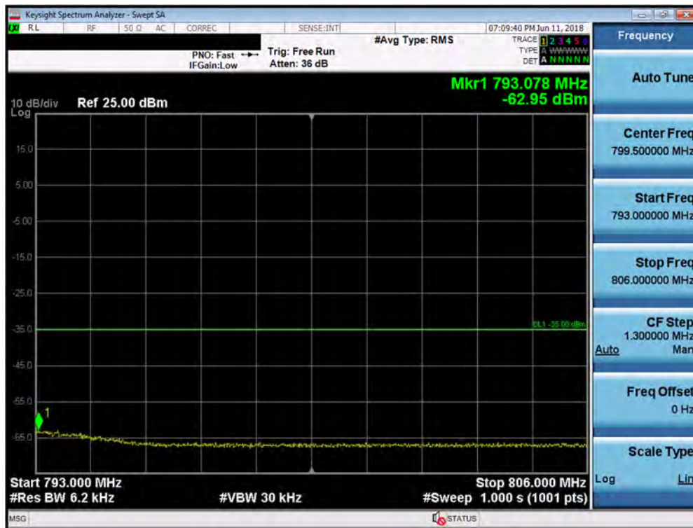
Plot 7-177. Upper Emission Mask Edge Plot (Band 13 – 5.0MHz QPSK – Full RB Configuration)
