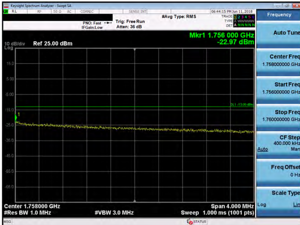
Plot 7-207. Upper Extended Band Edge Plot (Band 4 - 10.0MHz QPSK - Full RB Configuration)
