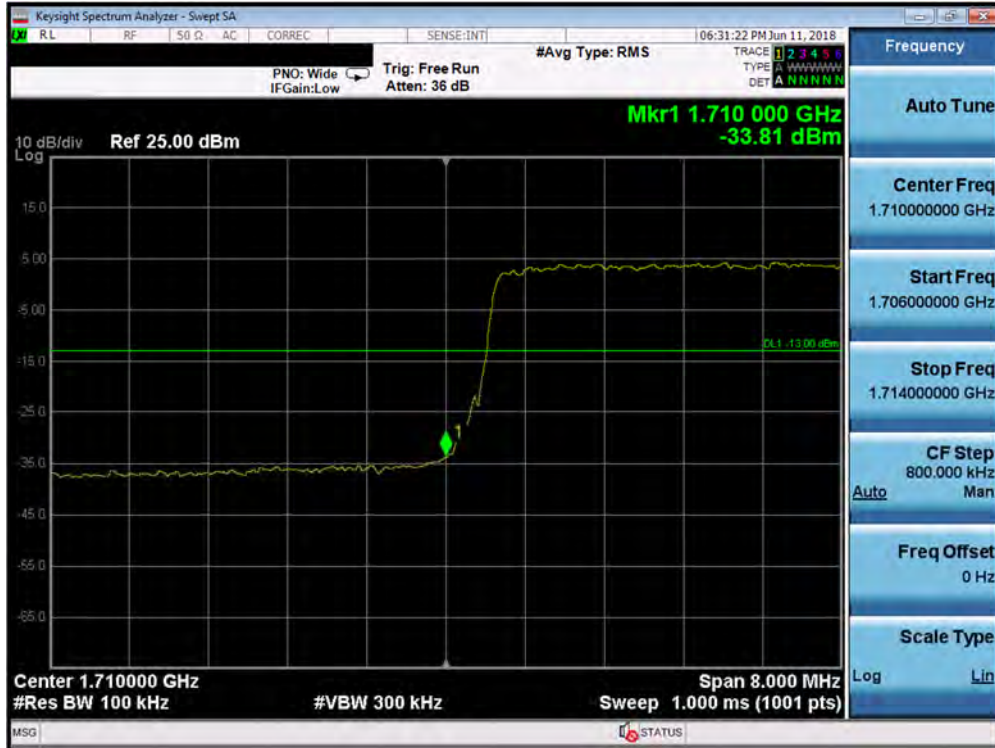
Plot 7-204. Lower Band Edge Plot (Band 4 - 10.0MHz QPSK - Full RB Configuration)
