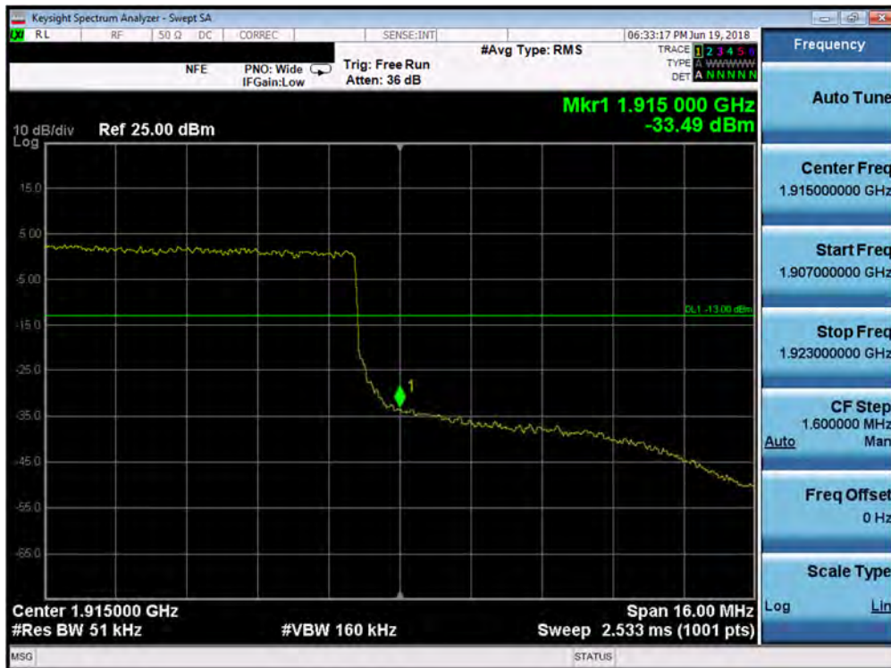
Plot 7-250. Upper Band Edge Plot (Band 25 - 20.0MHz QPSK - Full RB Configuration)
