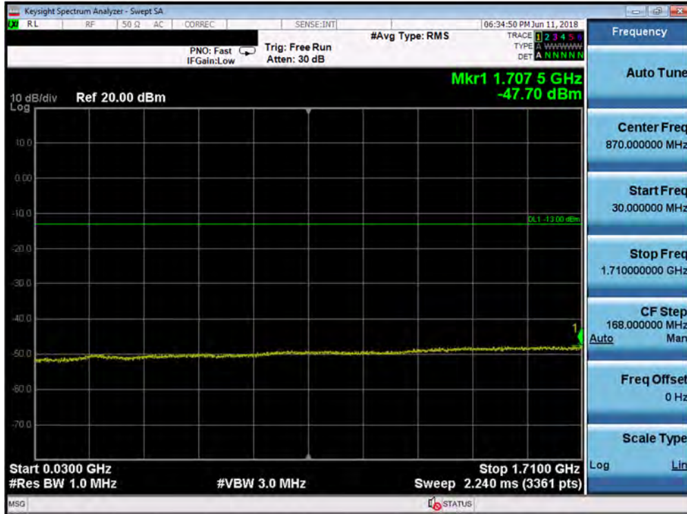
Plot 7-136. Conducted Spurious Plot (Band 4 - 5.0MHz QPSK - RB Size 1, RB Offset 0 - High Channel)
