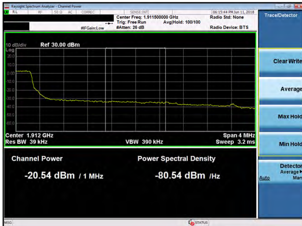
Plot 7-231. Upper Extended Band Edge Plot (Band 2 - 5.0MHz QPSK - Full RB Configuration)
