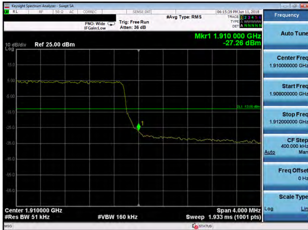
Plot 7-230. Upper Band Edge Plot (Band 2 - 5.0MHz QPSK - Full RB Configuration)
