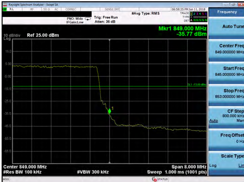
Plot 7-189. Upper Band Edge Plot (Band 26/5 - 10.0MHz QPSK - Full RB Configuration)
