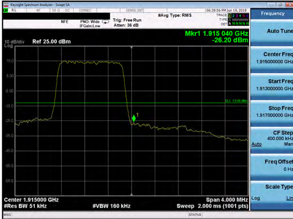
Plot 7-220. Upper Band Edge Plot (Band 25 - 1.4MHz QPSK - Full RB Configuration)
