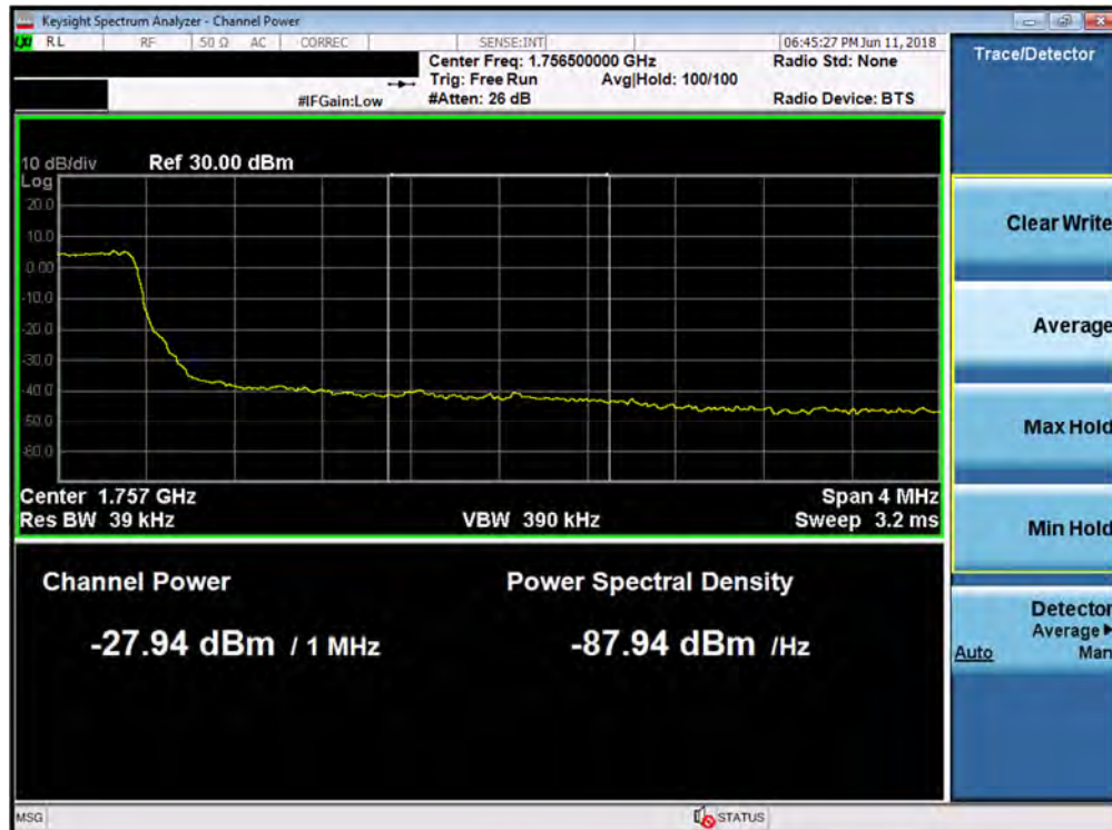
Plot 7-199. Upper Extended Band Edge Plot (Band 4 - 3.0MHz QPSK - Full RB Configuration)
