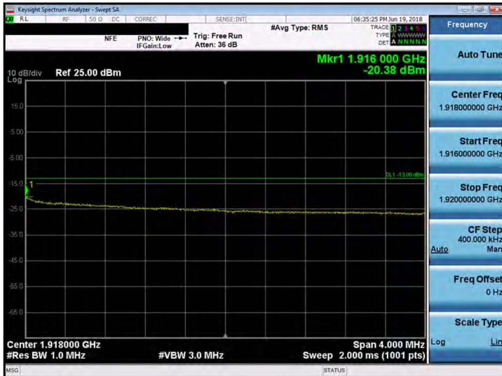
Plot 7-239. Upper Extended Band Edge Plot (Band 25 - 10.0MHz QPSK - Full RB Configuration)
