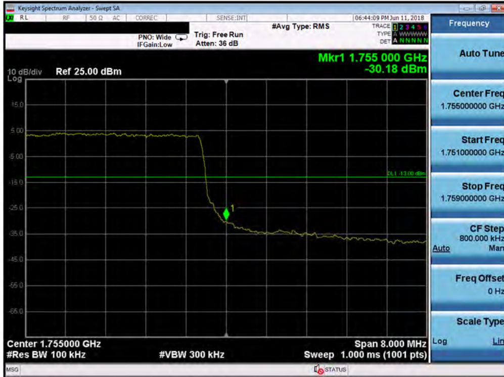
Plot 7-206. Upper Band Edge Plot (Band 4 - 10.0MHz QPSK - Full RB Configuration)
