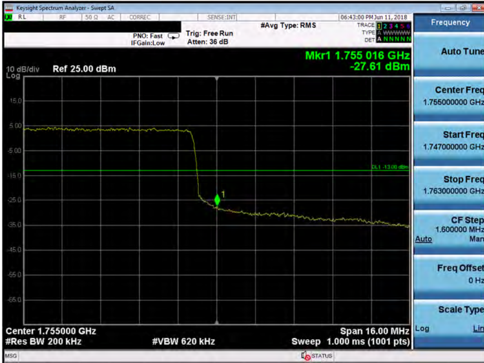
Plot 7-214. Upper Band Edge Plot (Band 4 - 20.0MHz QPSK - Full RB Configuration)
