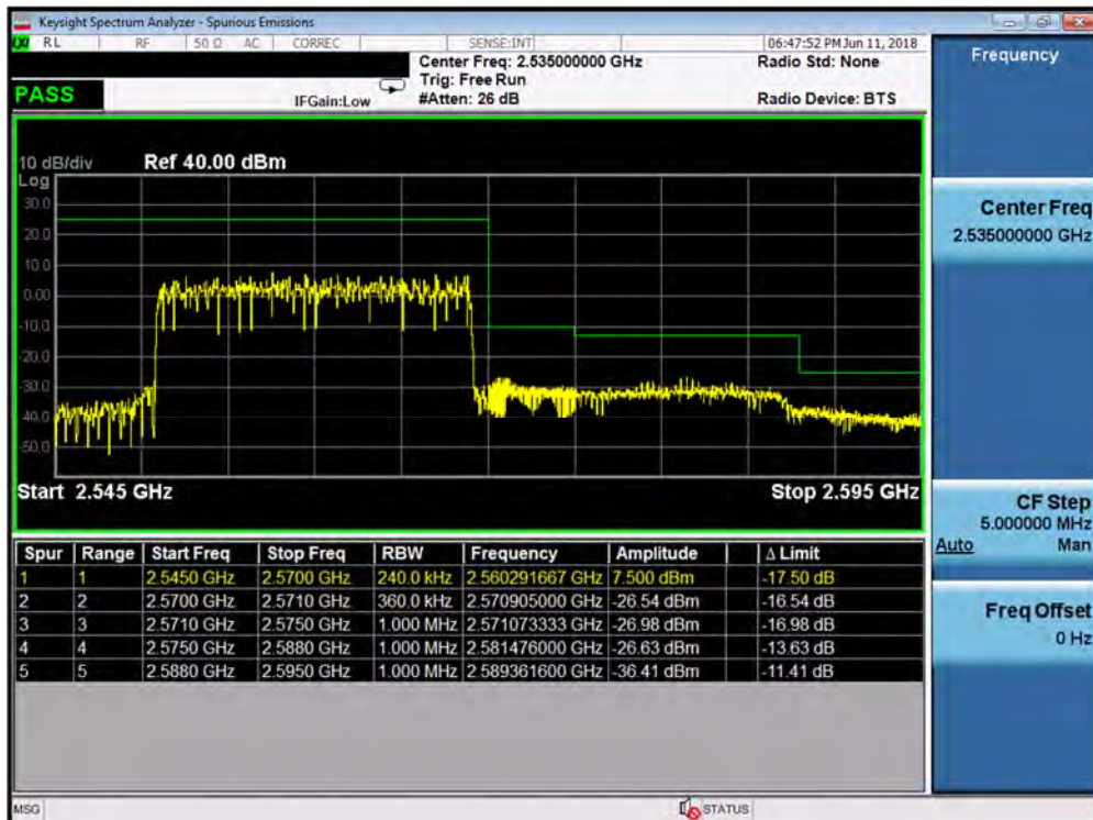
Plot 7-259. Upper Band Edge Plot (Band 7 - 20.0MHz QPSK - Full RB Configuration)
