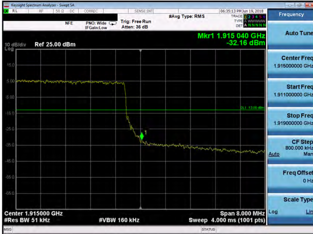
Plot 7-238. Upper Band Edge Plot (Band 25 - 10.0MHz QPSK - Full RB Configuration)
