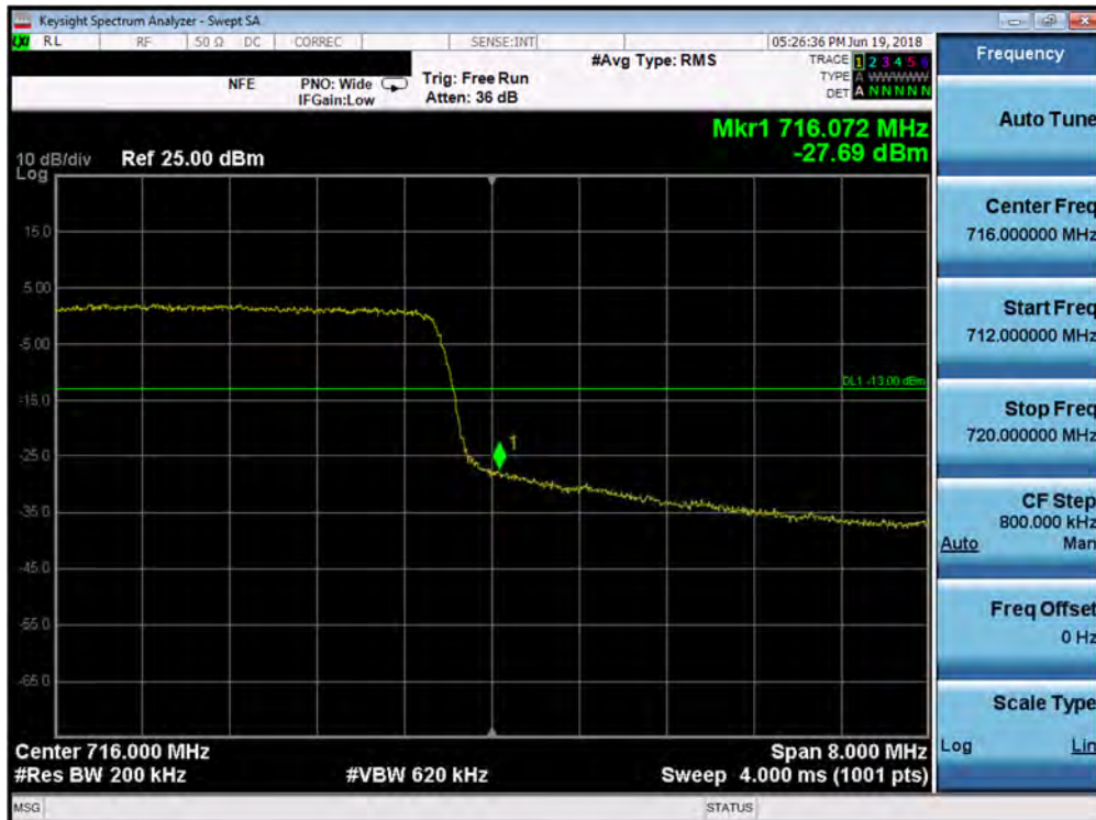
Plot 7-173. Upper Band Edge Plot (Band 12 - 10.0MHz QPSK - Full RB Configuration)
