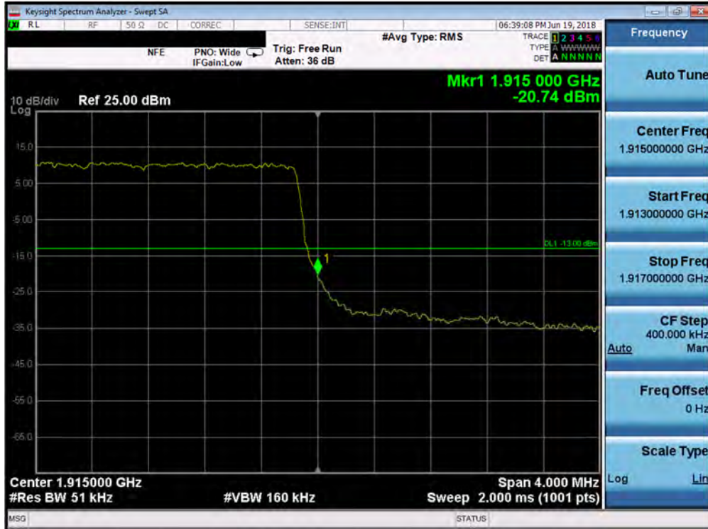
Plot 7-226. Upper Band Edge Plot (Band 25 - 3.0MHz QPSK - Full RB Configuration)
