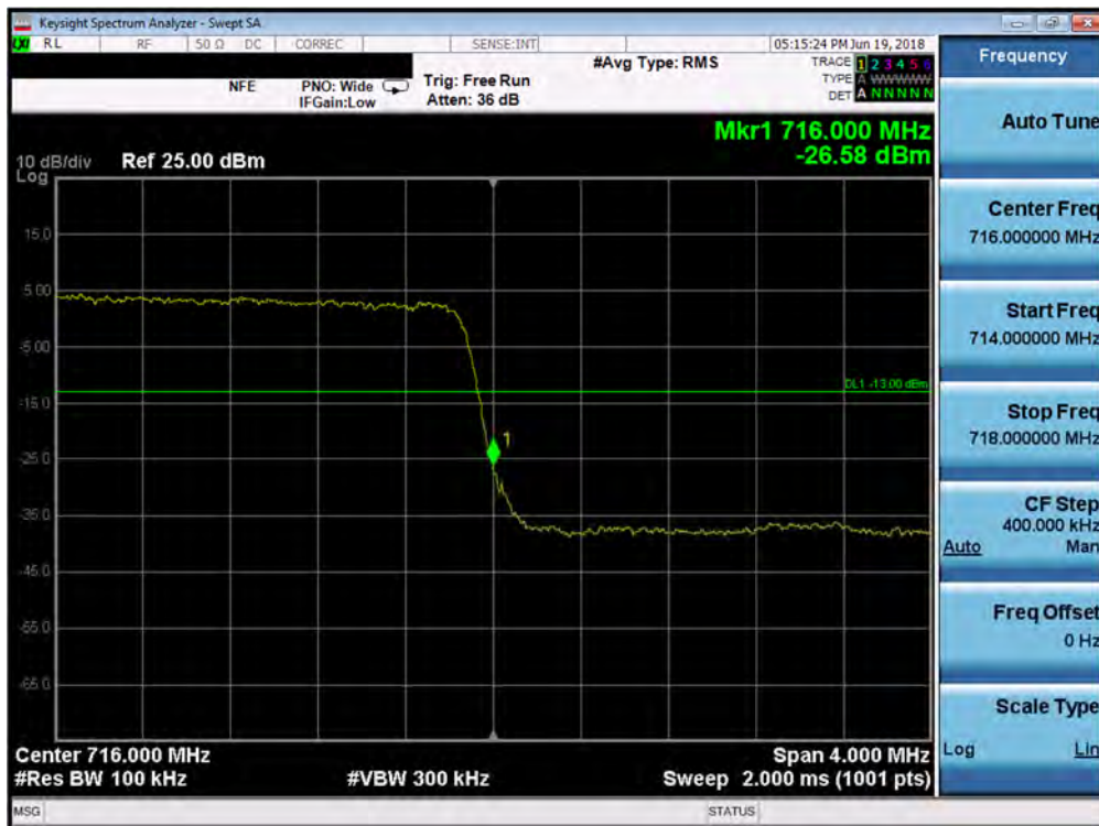
Plot 7-169. Upper Band Edge Plot (Band 12 - 3.0MHz QPSK - Full RB Configuration)
