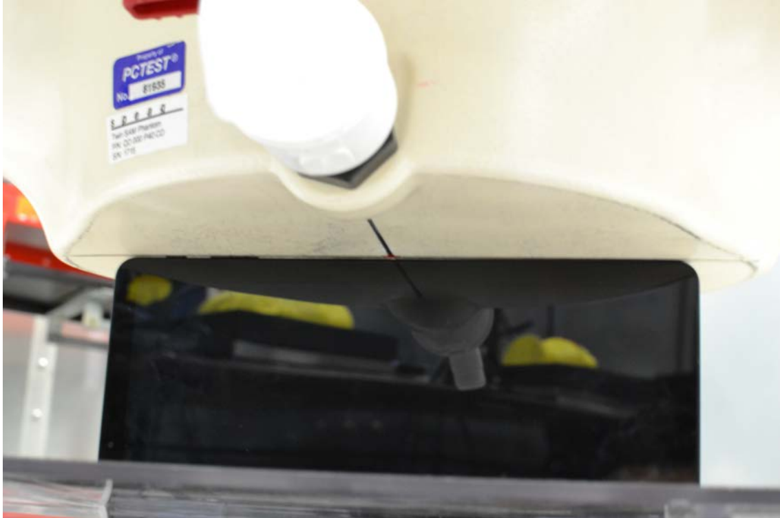
SAR Test Setup Photo 9 – Right Edge at 0.0 cm (Licensed and Unlicensed Modes)
