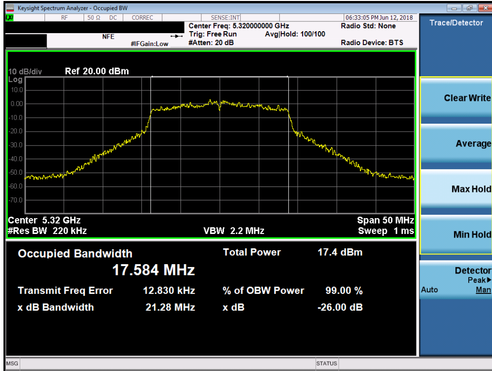
Plot 7-15. 26dB Bandwidth Plot (20MHz BW 802.11n (UNII Band 2A) – Ch. 64)
