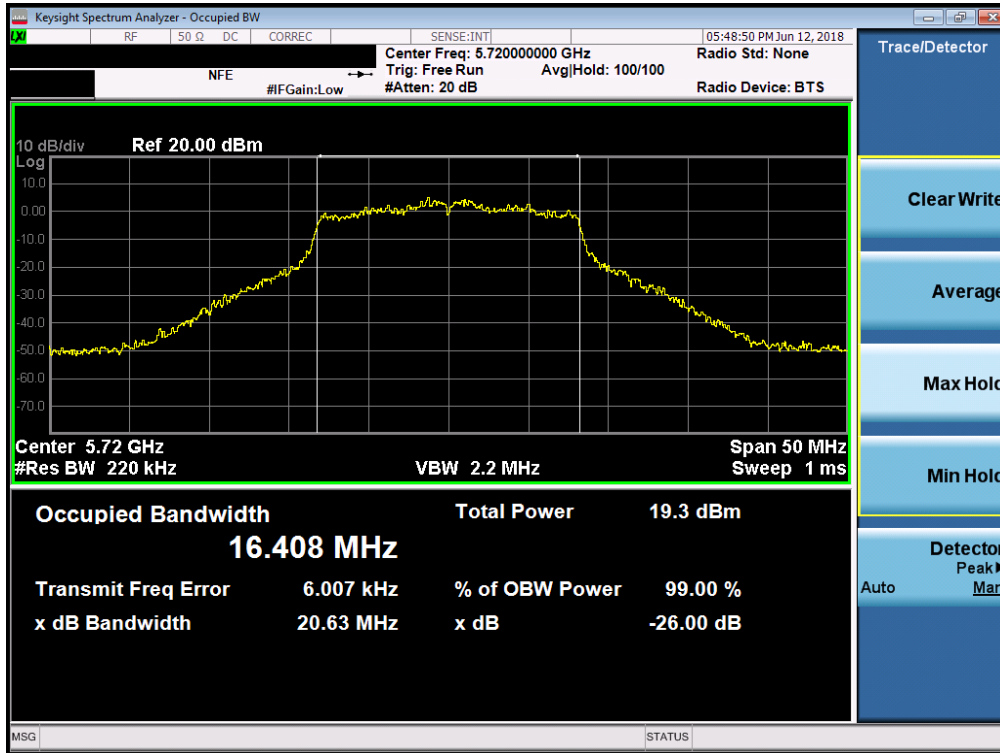
Plot 7-51. 26dB Bandwidth Plot (802.11a (UNII Band 2C) – Ch. 144)
