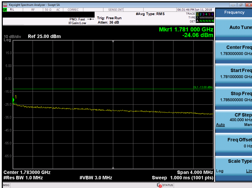
Plot 7-172. Upper Extended Band Edge Plot (Band 66 - 10.0MHz QPSK - Full RB Configuration)
