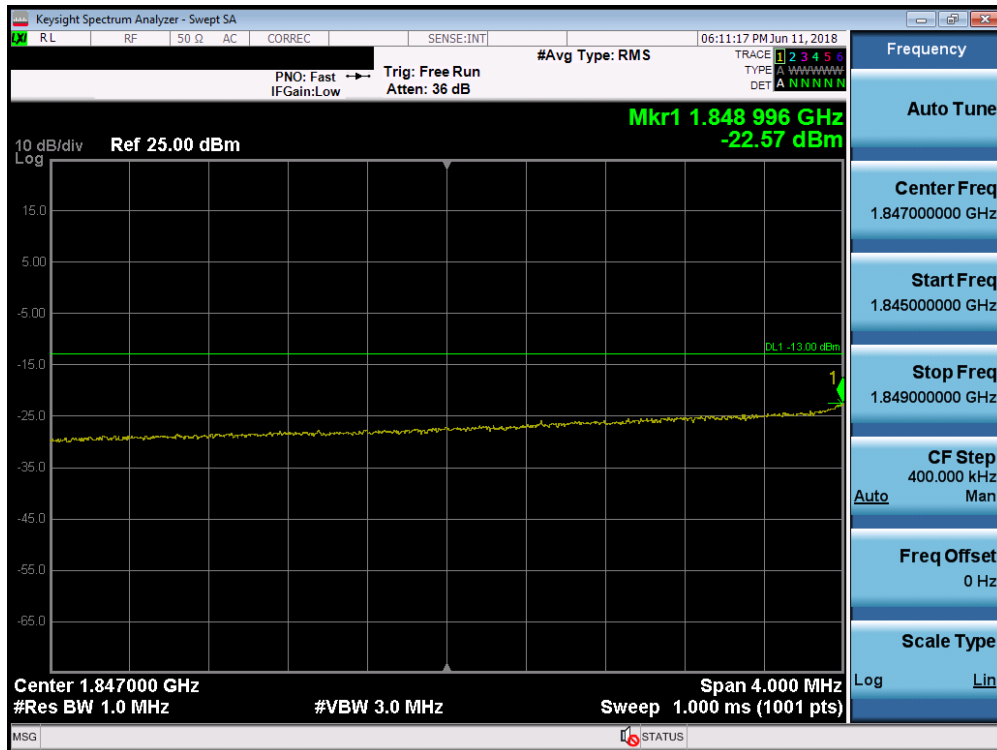
Plot 7-198. Lower Extended Band Edge Plot (Band 2 - 10.0MHz QPSK - Full RB Configuration)
