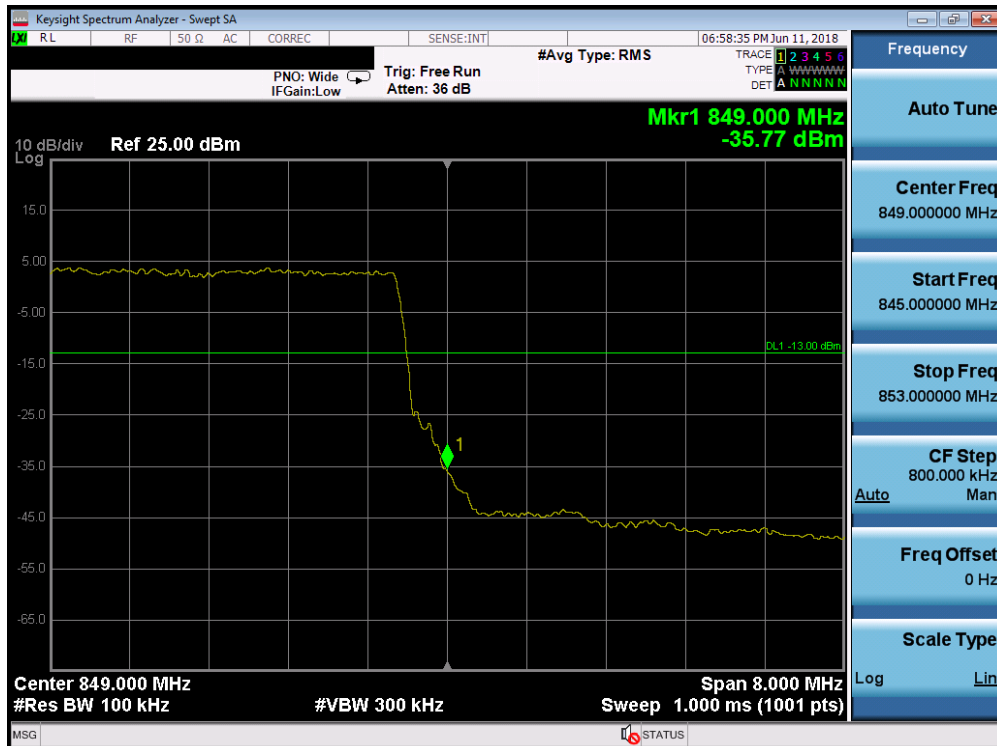
Plot 7-148. Upper Band Edge Plot (Band 5 - 10.0MHz QPSK - Full RB Configuration)
