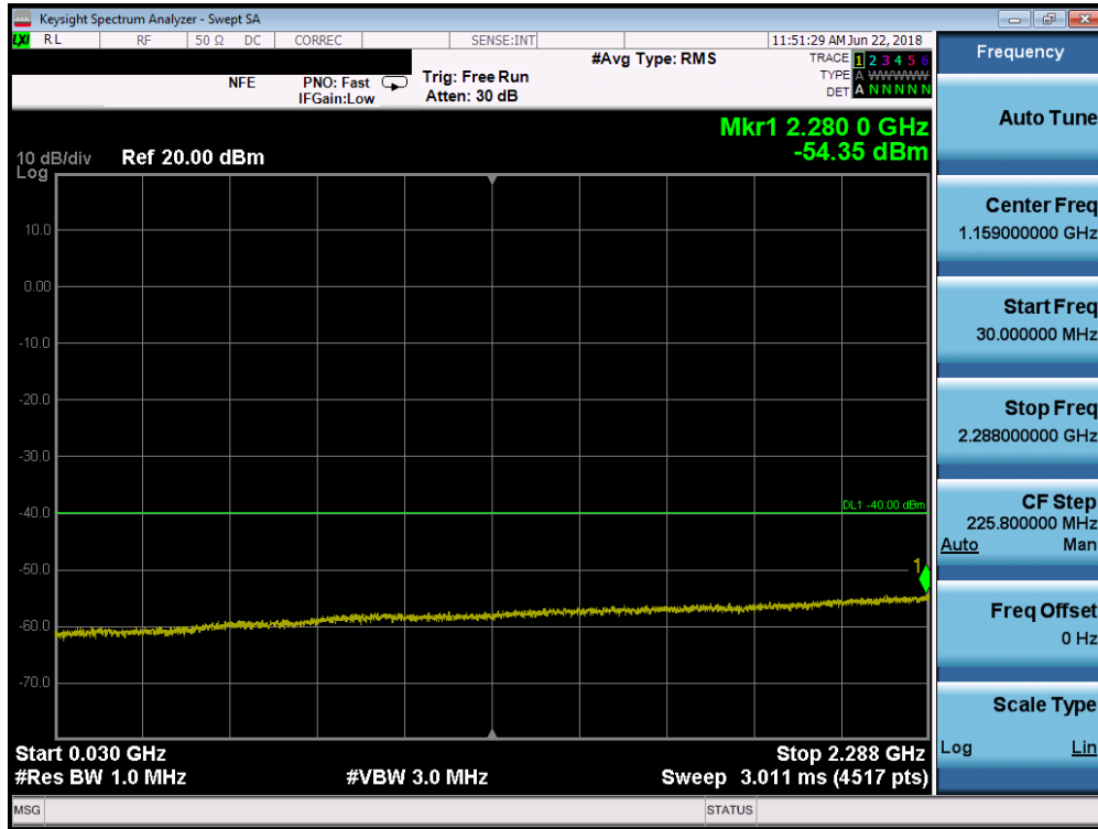
Plot 7-115. Conducted Spurious Plot (Band 30 - 5.0MHz QPSK - RB Size 1, RB Offset 0 - Low Channel)
