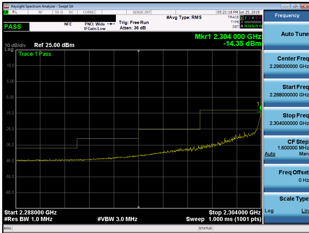
Plot 7-210. Lower Extended Band Edge Plot (Band 30 - 5.0MHz QPSK - Full RB Configuration)
