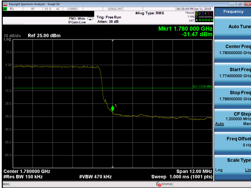
Plot 7-177. Upper Band Edge Plot (Band 66 - 15.0MHz QPSK - Full RB Configuration)
