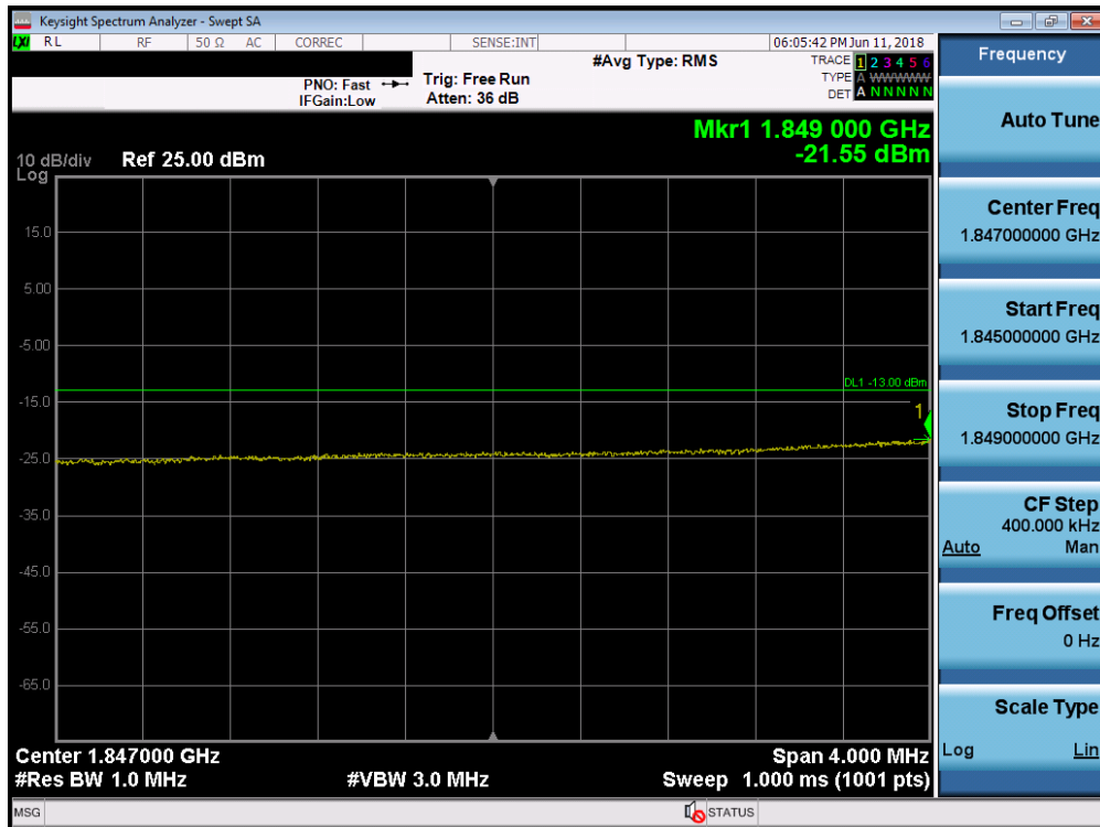
Plot 7-206. Lower Extended Band Edge Plot (Band 2 - 20.0MHz QPSK - Full RB Configuration)
