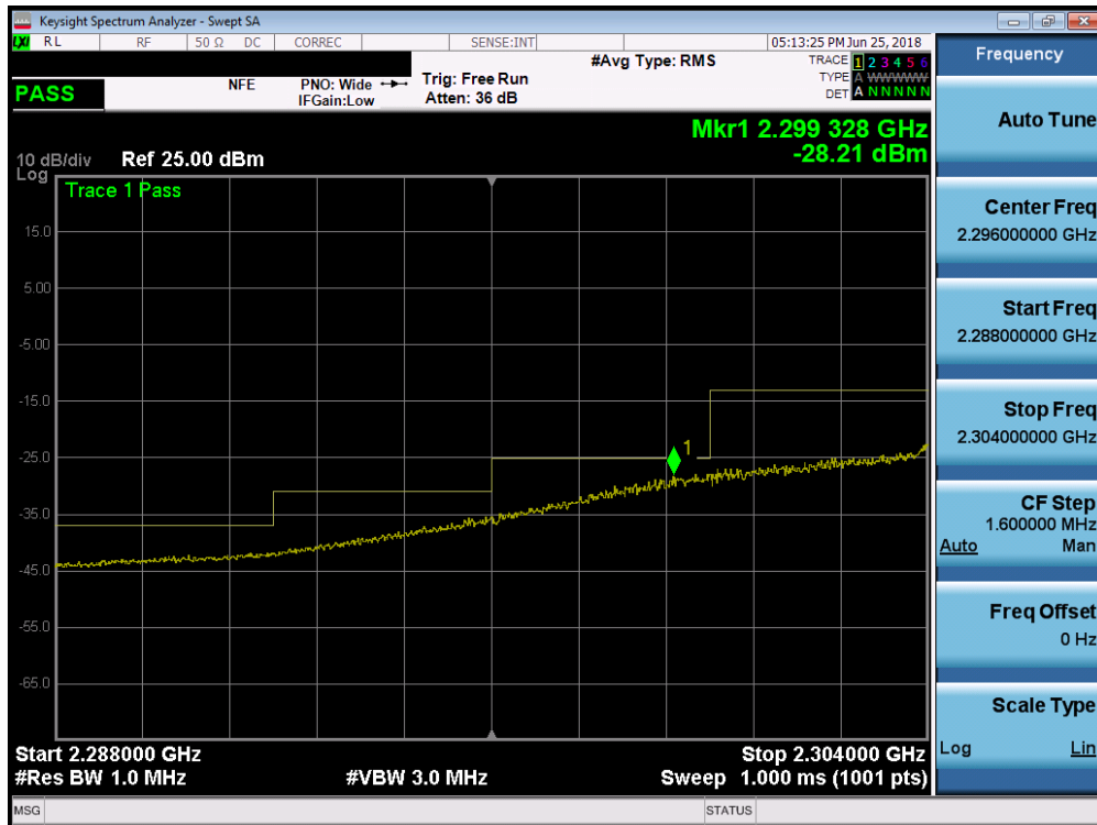
Plot 7-214. Lower Extended Band Edge Plot (Band 30 - 10.0MHz QPSK - Full RB Configuration)
