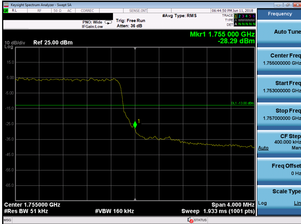
Plot 7-163. Upper Band Edge Plot (Band 4 - 5.0MHz QPSK - Full RB Configuration)
