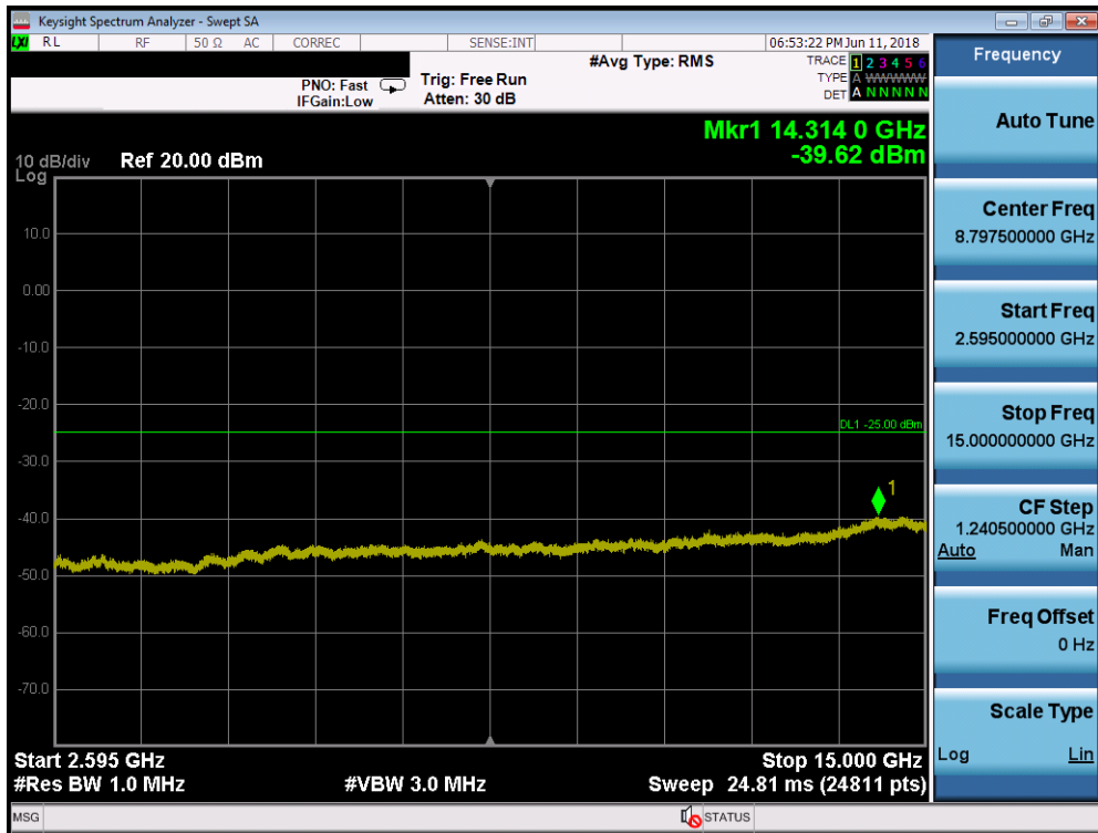
Plot 7-131. Conducted Spurious Plot (Band 7 - 5.0MHz QPSK - RB Size 1, RB Offset 0 - High Channel)
