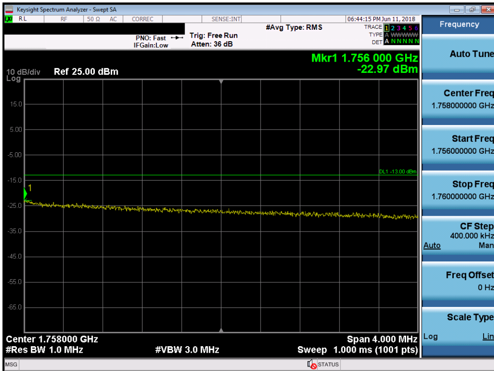
Plot 7-170. Upper Extended Band Edge Plot (Band 4 - 10.0MHz QPSK - Full RB Configuration)
