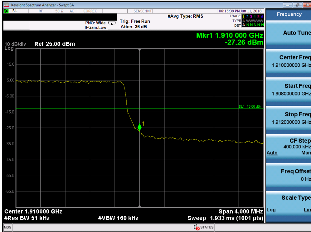
Plot 7-195. Upper Band Edge Plot (Band 2 - 5.0MHz QPSK - Full RB Configuration)
