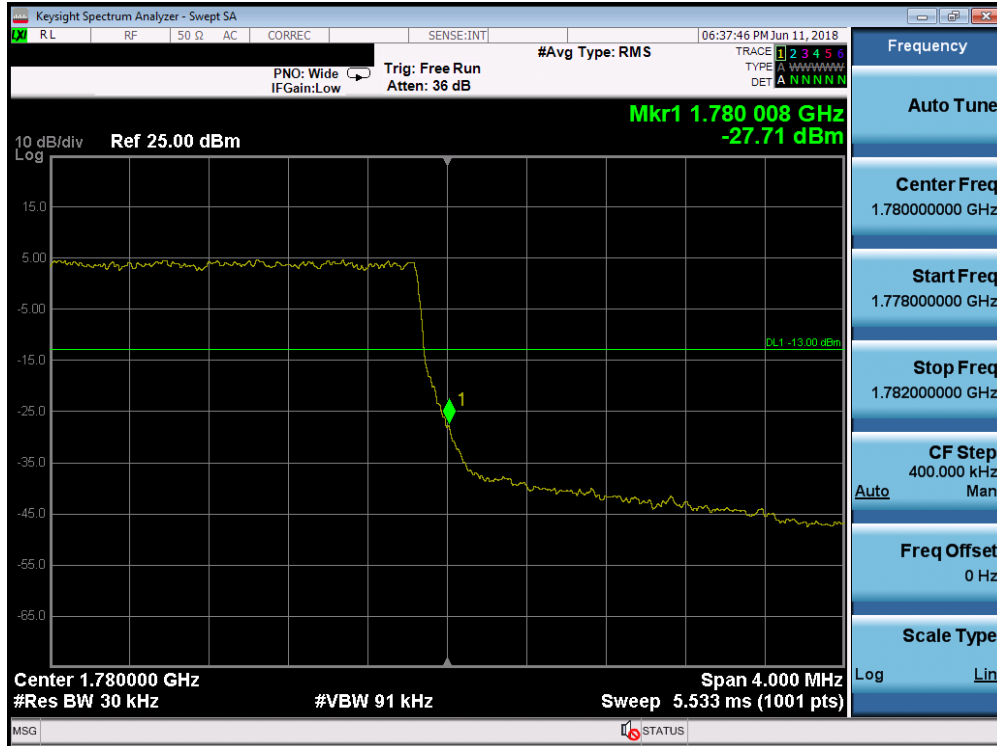
Plot 7-159. Upper Band Edge Plot (Band 66 - 3.0MHz QPSK - Full RB Configuration)
