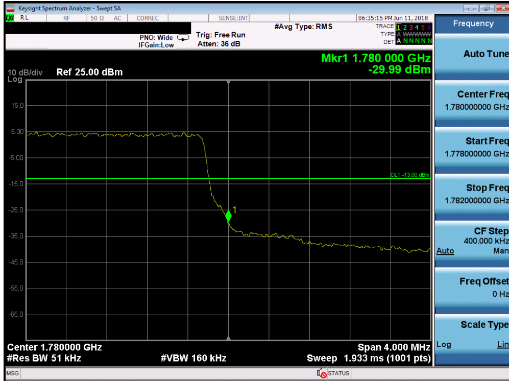
Plot 7-165. Upper Band Edge Plot (Band 66 - 5.0MHz QPSK - Full RB Configuration)
