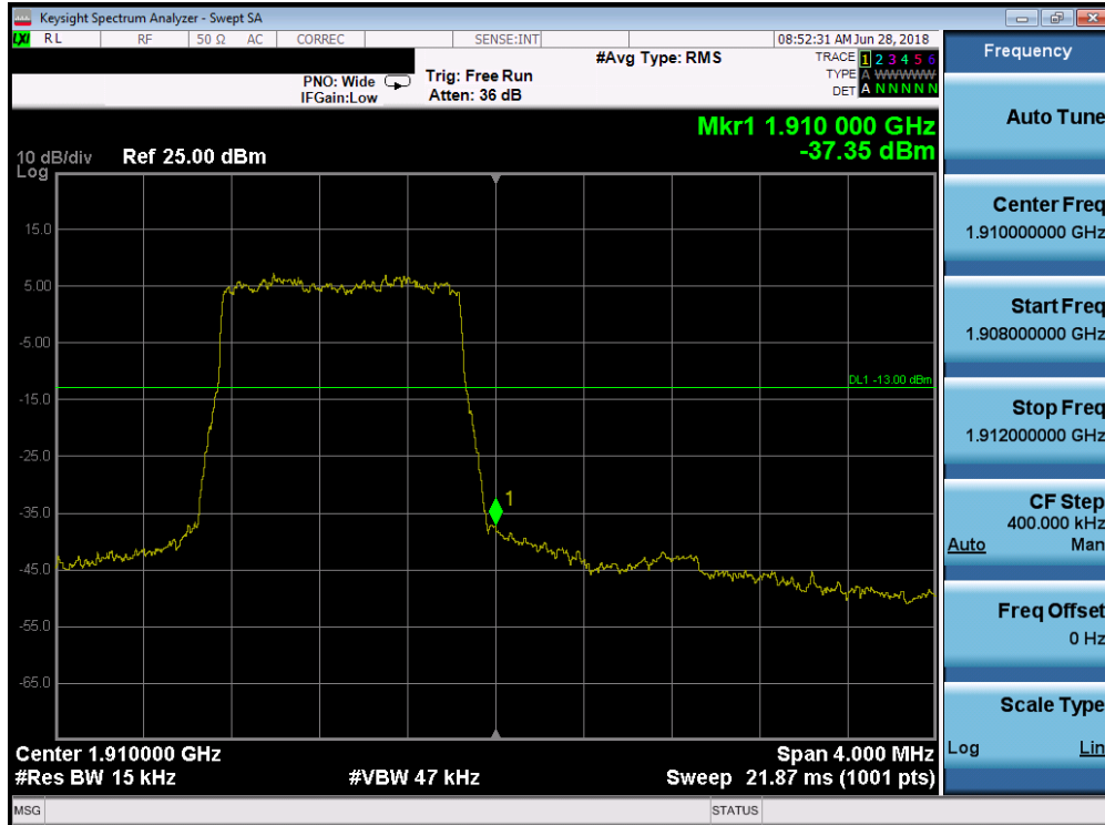
Plot 7-187. Upper Band Edge Plot (Band 2 - 1.4MHz QPSK - Full RB Configuration)
