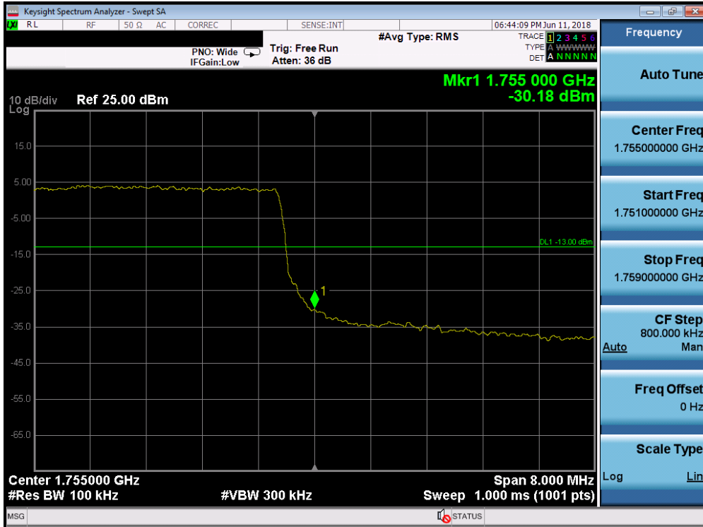
Plot 7-169. Upper Band Edge Plot (Band 4 - 10.0MHz QPSK - Full RB Configuration)
