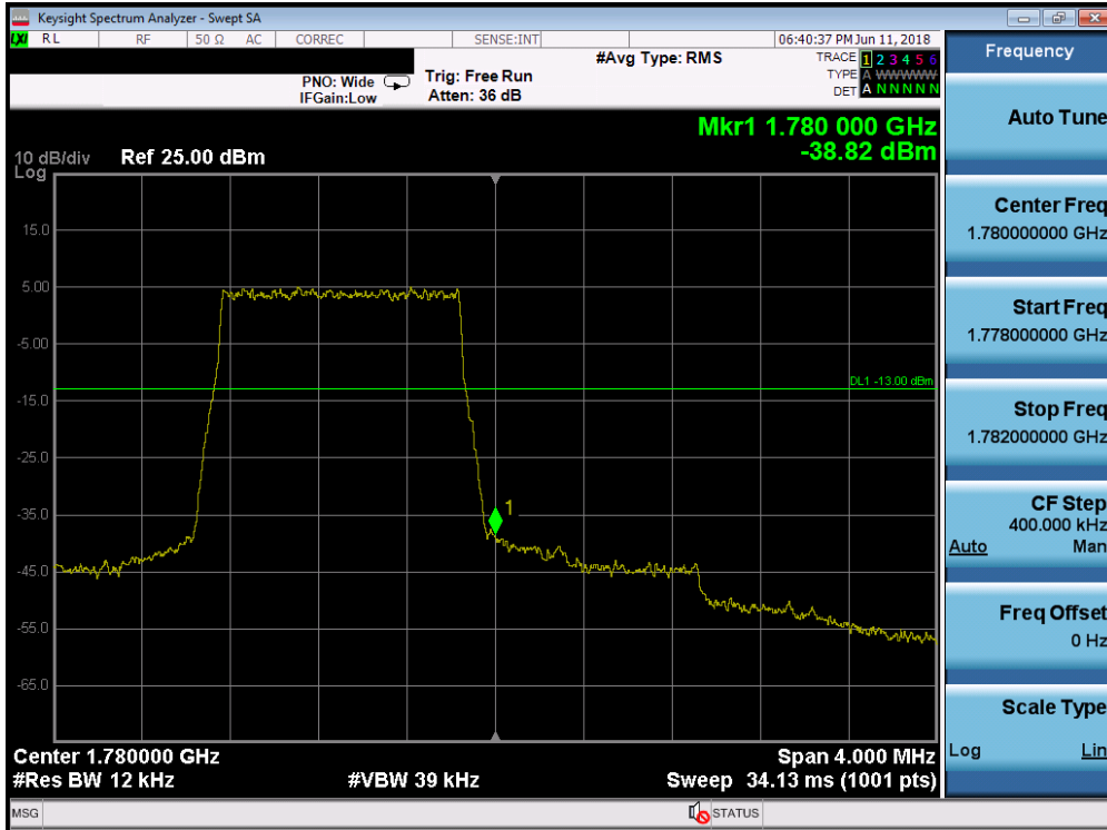
Plot 7-153. Upper Band Edge Plot (Band 66 - 1.4MHz QPSK - Full RB Configuration)
