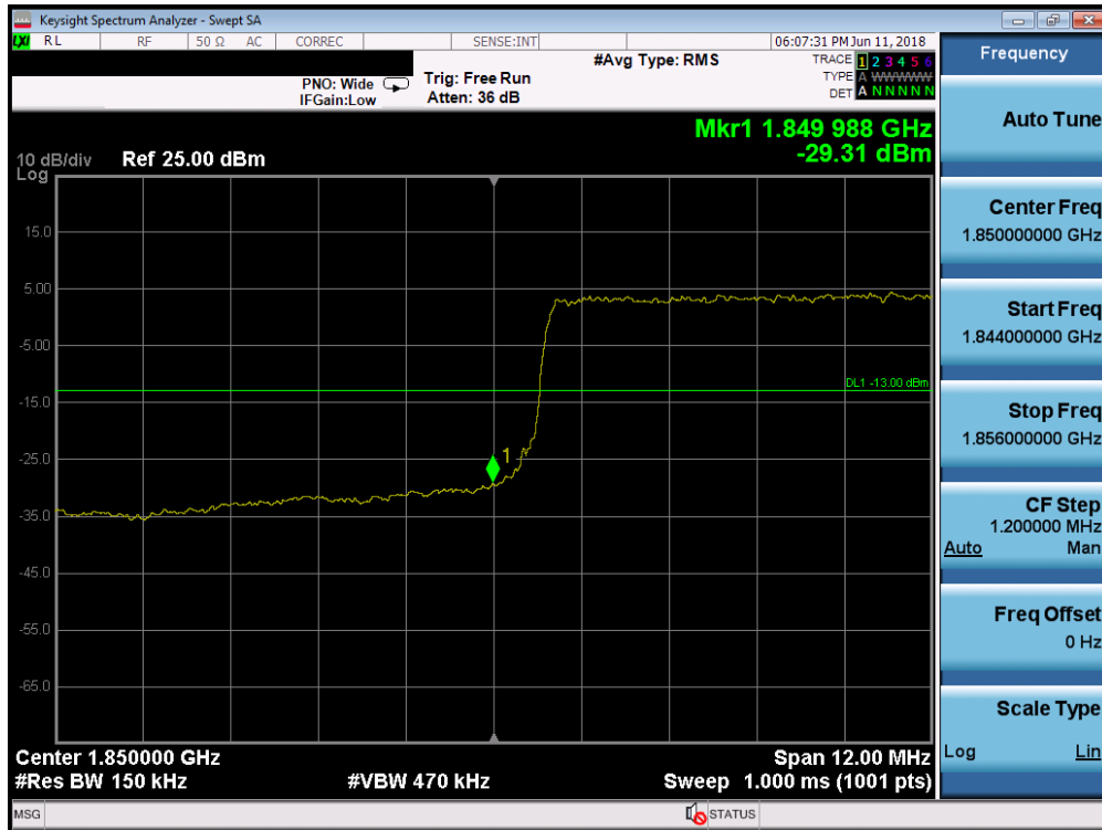
Plot 7-201. Lower Band Edge Plot (Band 2 - 15.0MHz QPSK - Full RB Configuration)
