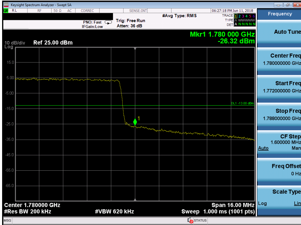
Plot 7-183. Upper Band Edge Plot (Band 66 - 20.0MHz QPSK - Full RB Configuration)
