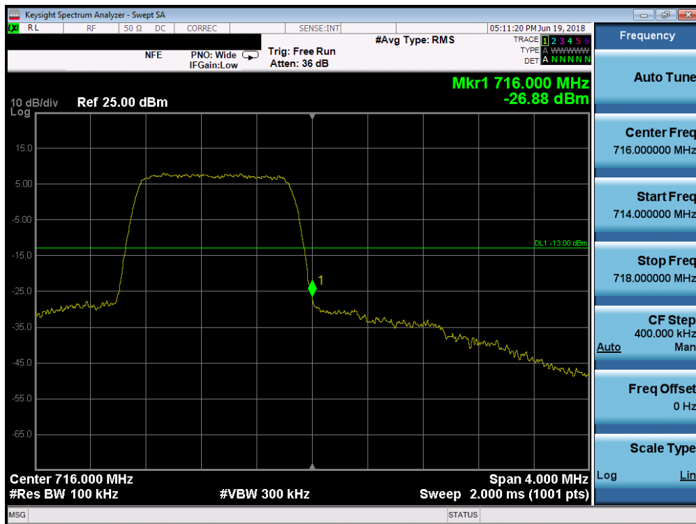
Plot 7-134. Upper Band Edge Plot (Band 12 - 1.4MHz QPSK - Full RB Configuration)
