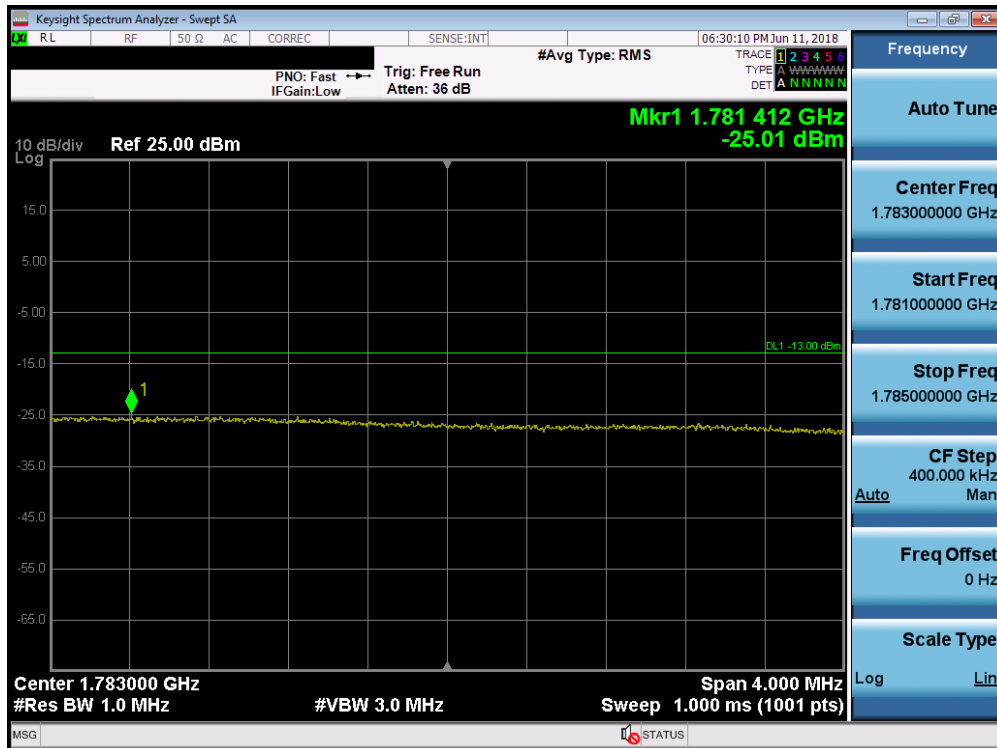
Plot 7-178. Upper Extended Band Edge Plot (Band 66 - 15.0MHz QPSK - Full RB Configuration)
