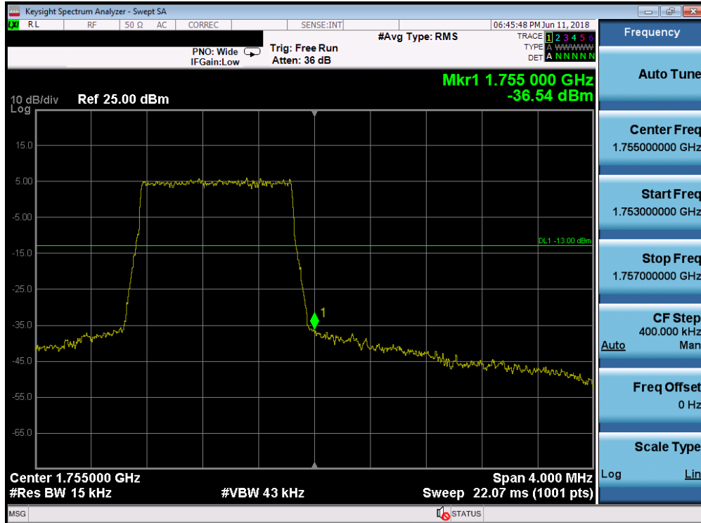
Plot 7-151. Upper Band Edge Plot (Band 4 - 1.4MHz QPSK - Full RB Configuration)
