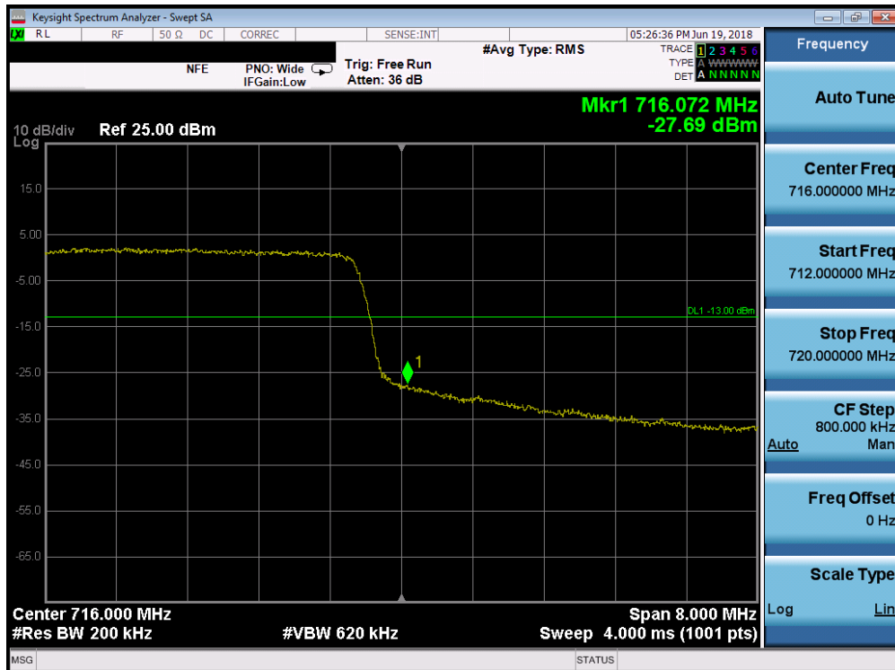
Plot 7-140. Upper Band Edge Plot (Band 12 - 10.0MHz QPSK - Full RB Configuration)
