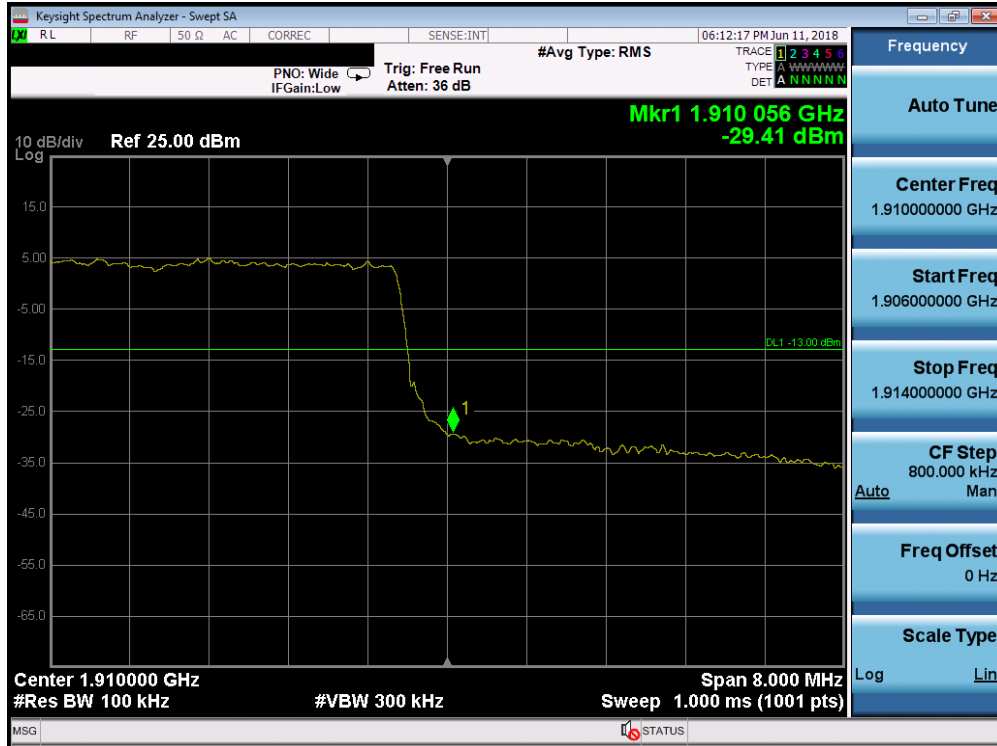
Plot 7-199. Upper Band Edge Plot (Band 2 - 10.0MHz QPSK - Full RB Configuration)
