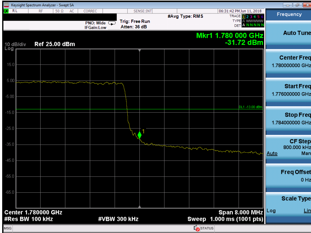
Plot 7-171. Upper Band Edge Plot (Band 66 - 10.0MHz QPSK - Full RB Configuration)
