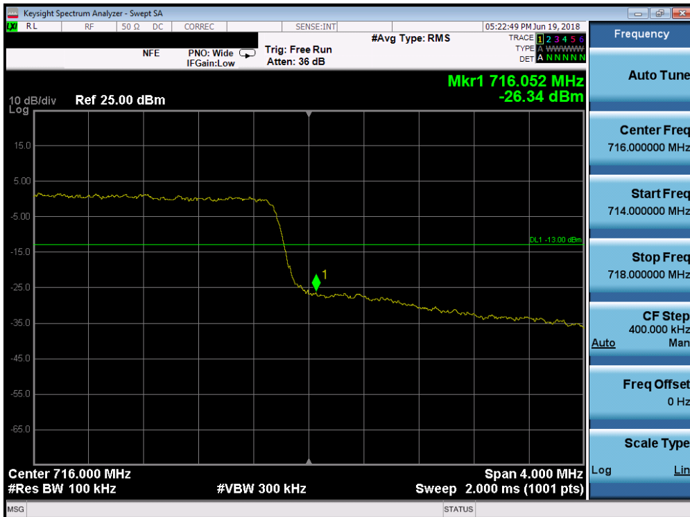
Plot 7-138. Upper Band Edge Plot (Band 12 - 5.0MHz QPSK - Full RB Configuration)
