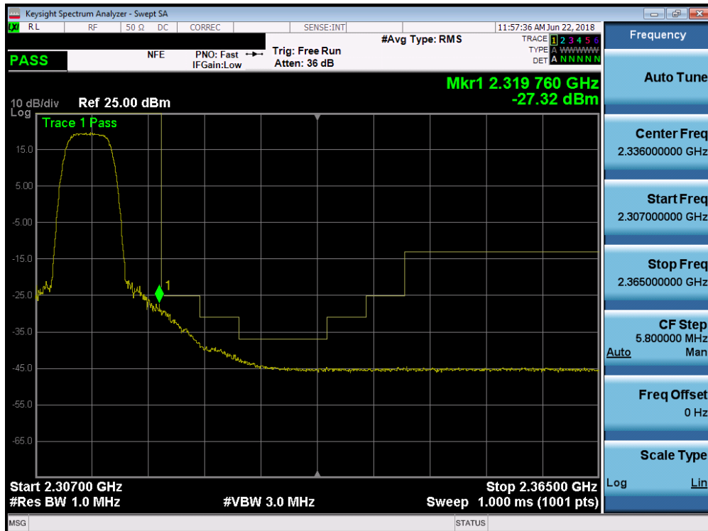
Plot 7-212. Upper Extended Band Edge Plot (Band 30 - 5.0MHz QPSK - Full RB Configuration)
