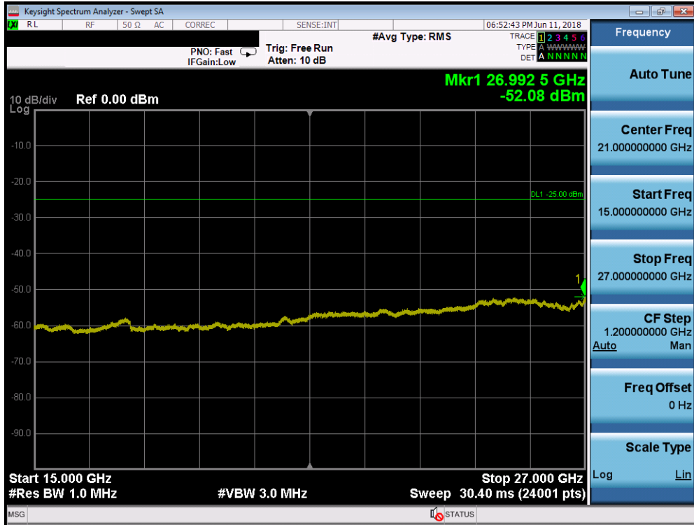
Plot 7-126. Conducted Spurious Plot (Band 7 - 5.0MHz QPSK - RB Size 1, RB Offset 0 - Low Channel)
