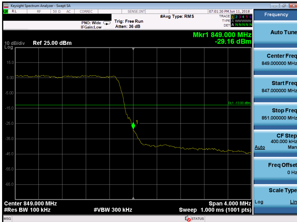
Plot 7-146. Upper Band Edge Plot (Band 5 - 5.0MHz QPSK - Full RB Configuration)
