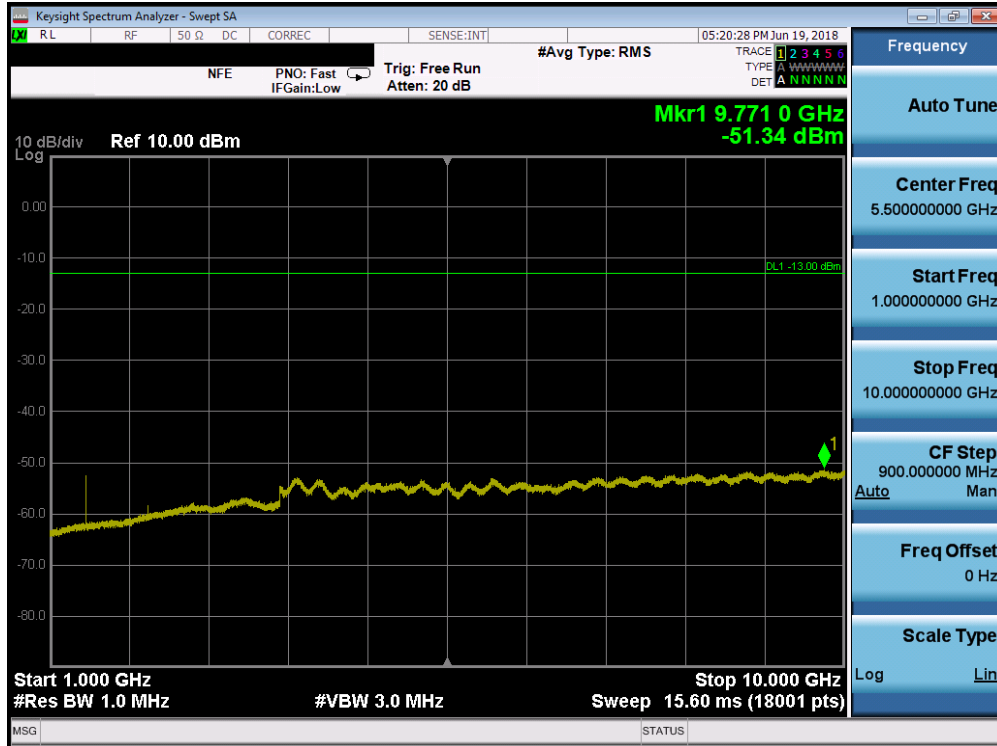
Plot 7-81. Conducted Spurious Plot (Band 12 - 5.0MHz QPSK - RB Size 1, RB Offset 0 - Low Channel)
