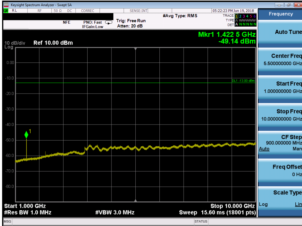
Plot 7-87. Conducted Spurious Plot (Band 12 - 5.0MHz QPSK - RB Size 1, RB Offset 0 - High Channel)
