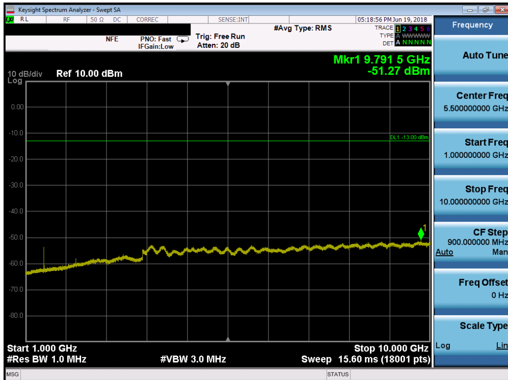
Plot 7-84. Conducted Spurious Plot (Band 12 - 5.0MHz QPSK - RB Size 1, RB Offset 0 - Mid Channel)
