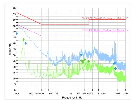
Note 1) Two graphs measured for both Live(L1) and Neutral(N) of the LISN are combined into one graph.
