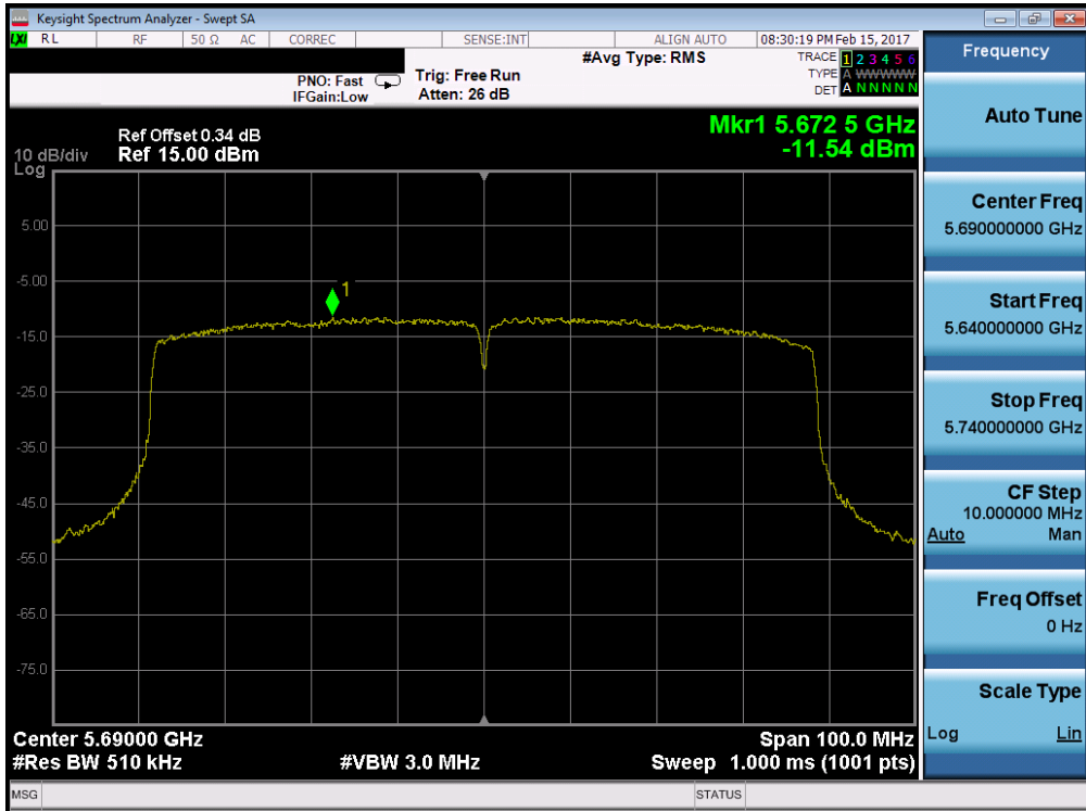
Plot 7-147. Power Spectral Density Plot (80MHz BW 802.11ac (UNII Band 2C) – Ch. 138)
