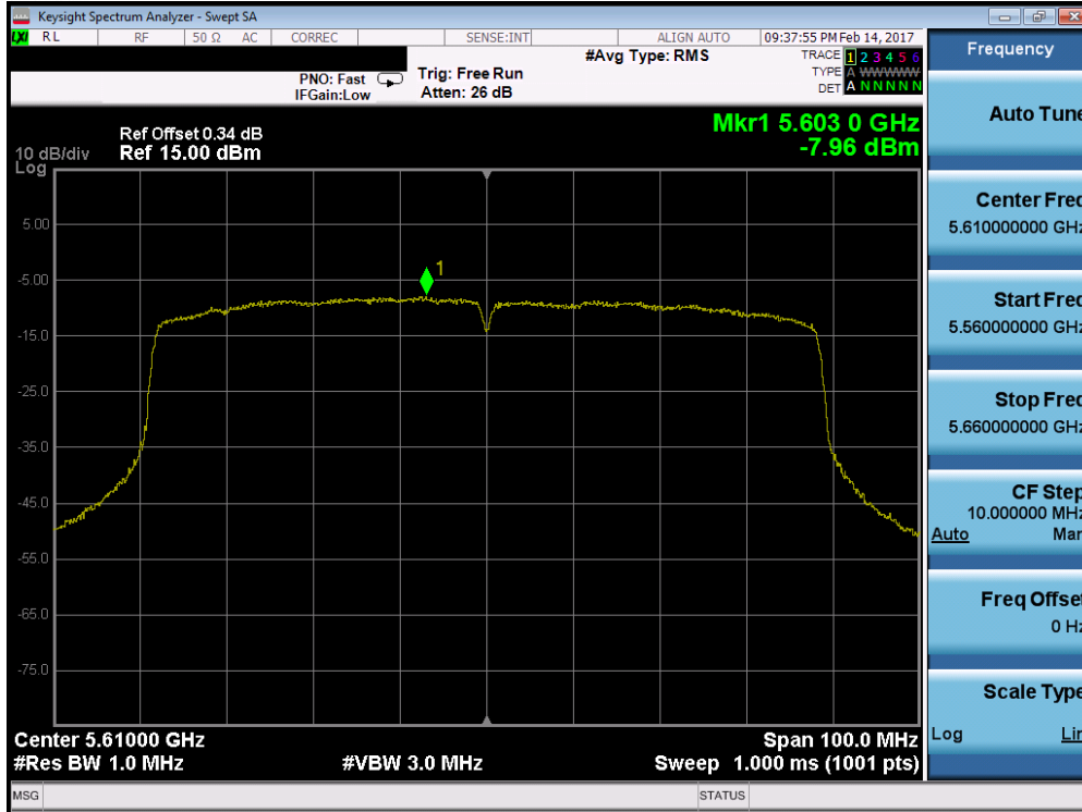
Plot 7-107. Power Spectral Density Plot (80MHz BW 802.11ac (UNII Band 2C) – Ch. 122)
