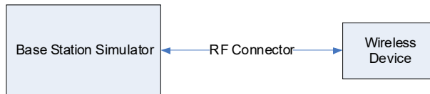
Figure 8-1 Power Measurement Setup
