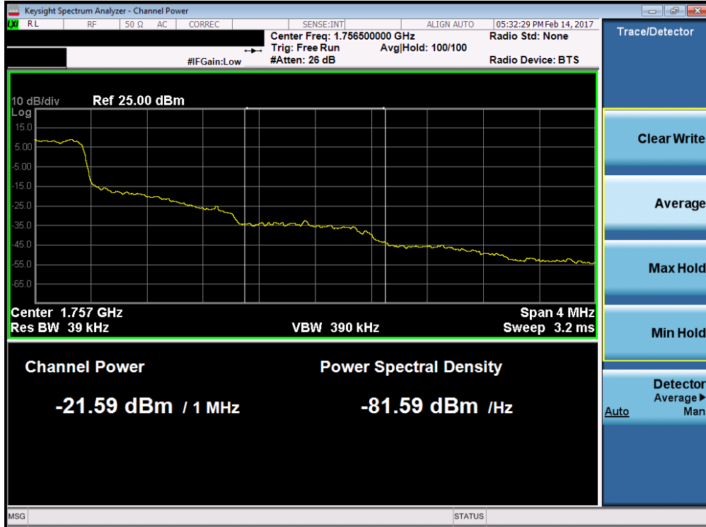
Plot 7-95. Upper Extended Band Edge Plot (Band 4 – 1.4MHz QPSK – RB Size 6)
