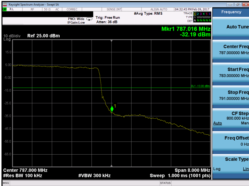
Plot 7-82. Upper Band Edge Plot (Band 13 – 10.0MHz QPSK – RB Size 50)
