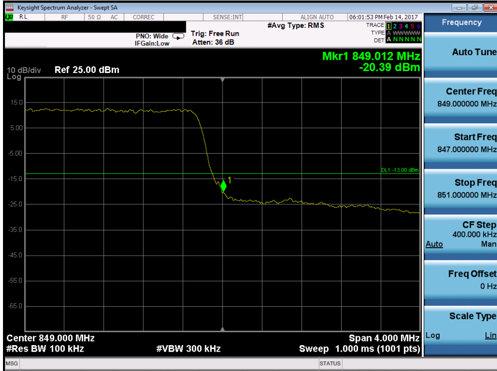
Plot 7-89. Upper Band Edge Plot (Band 5 – 5.0MHz QPSK – RB Size 25)
