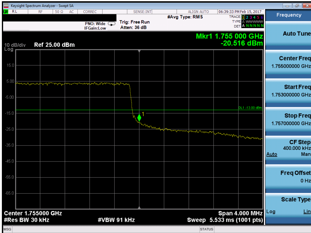
Plot 7-98. Upper Band Edge Plot (Band 4 – 3.0MHz QPSK – RB Size 15)
