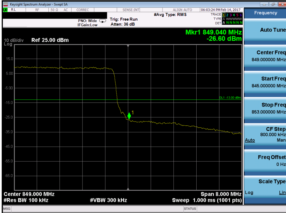
Plot 7-91. Upper Band Edge Plot (Band 5 – 10.0MHz QPSK – RB Size 50)
