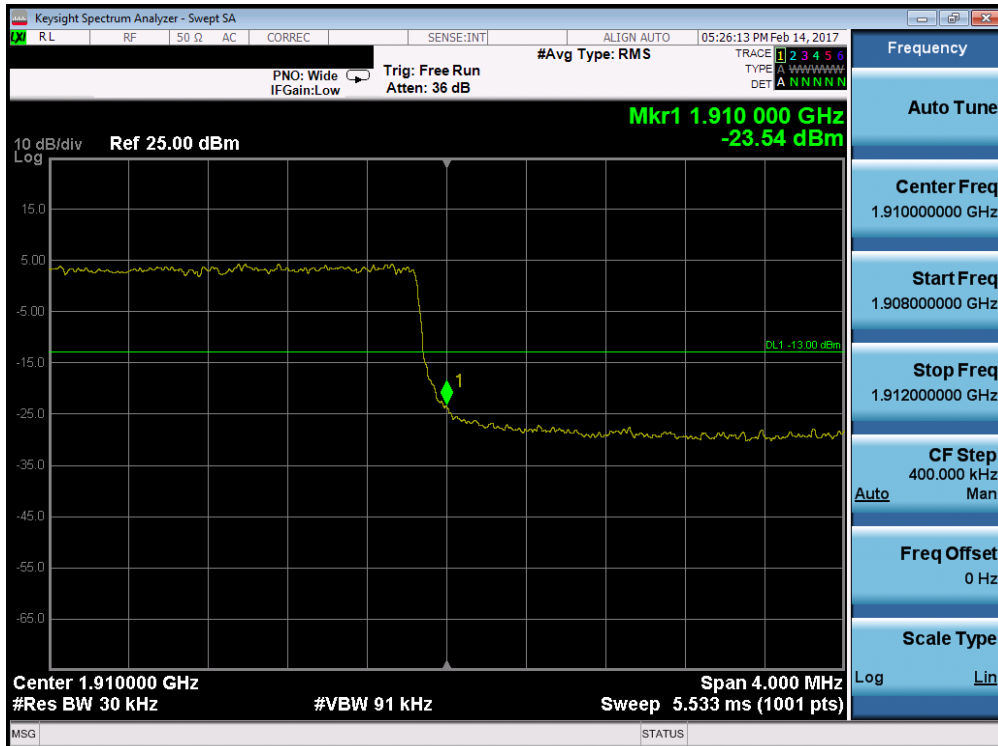
Plot 7-122. Upper Band Edge Plot (Band 2 – 3.0MHz QPSK – RB Size 15)
