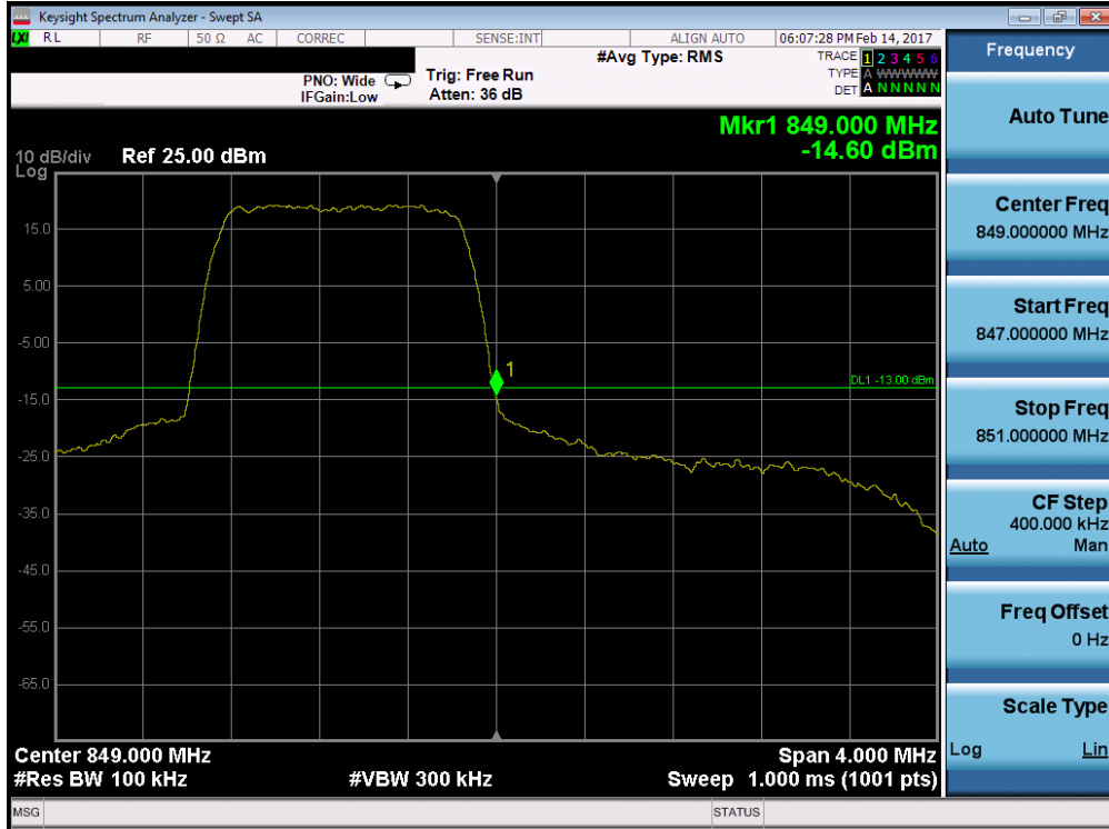
Plot 7-85. Upper Band Edge Plot (Band 5 – 1.4MHz QPSK – RB Size 6)
