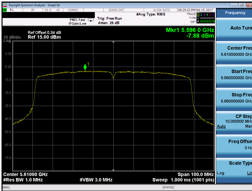
Plot 7-146. Power Spectral Density Plot (80MHz BW 802.11ac (UNII Band 2C) – Ch. 122)
