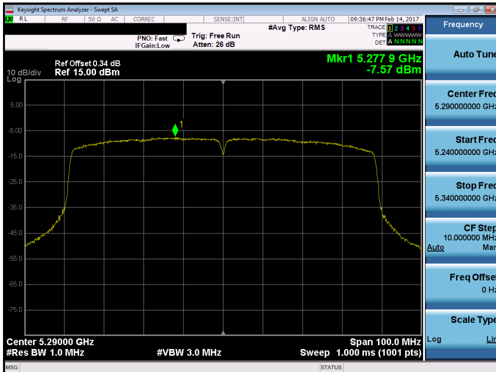
Plot 7-96. Power Spectral Density Plot (80MHz BW 802.11ac (UNII Band 2A) – Ch. 58)
