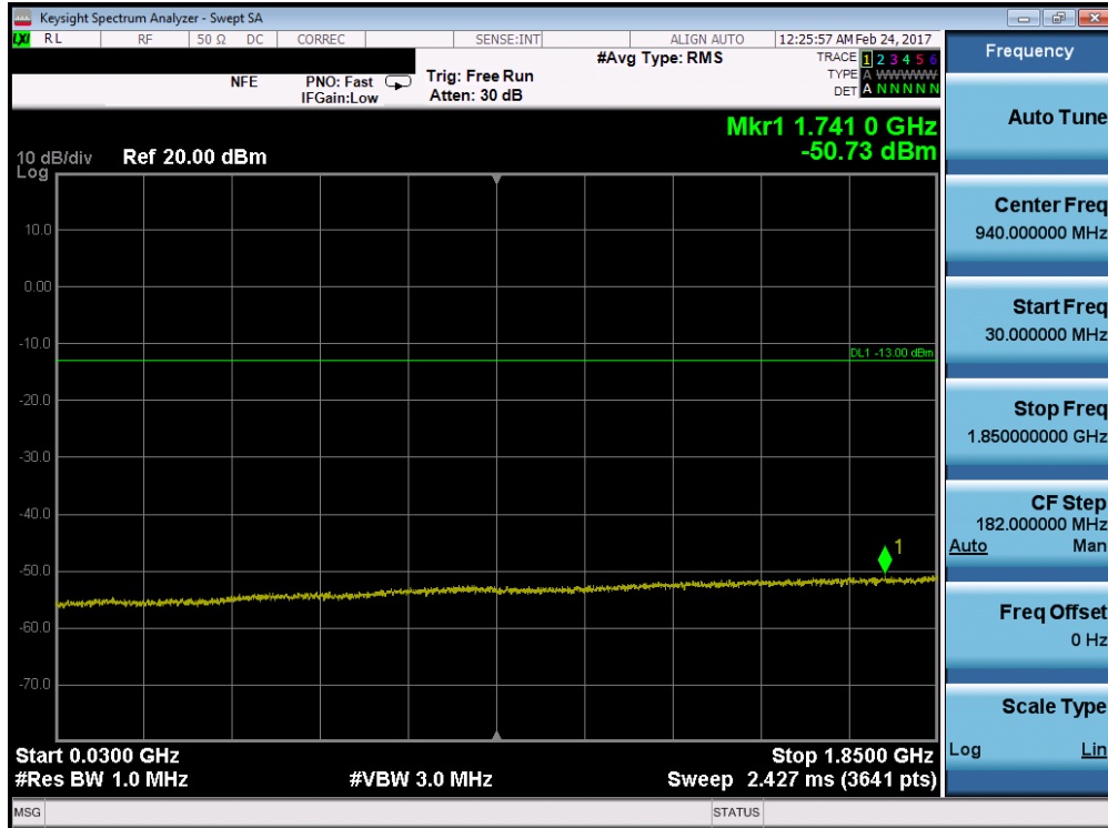
Plot 7-87. Conducted Spurious Plot (Band 25/2 – 3.0MHz QPSK – RB Size 1, RB Offset 0 – High Channel)
