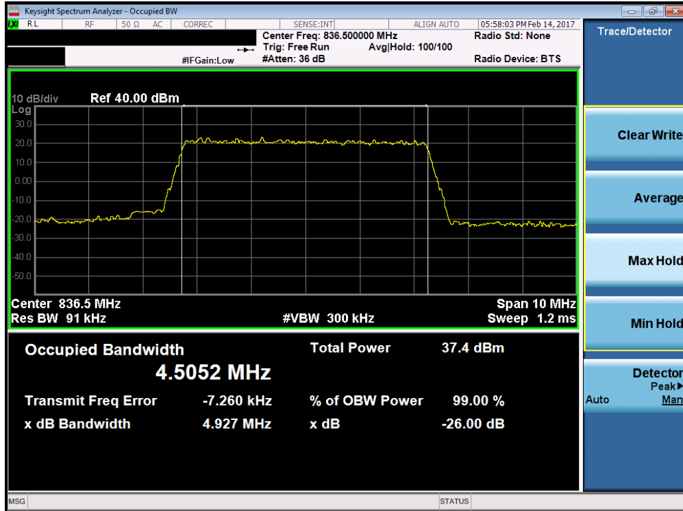
Plot 7-17. Occupied Bandwidth Plot (Band 5 – 5.0MHz QPSK – RB Size 25)
