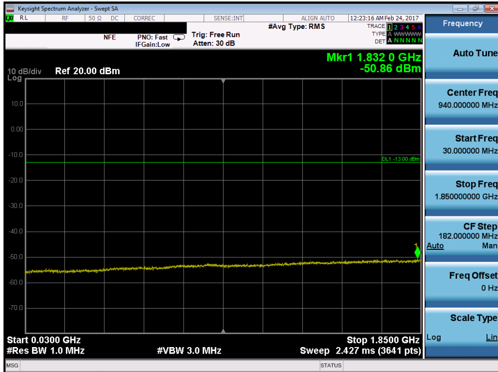
Plot 7-84. Conducted Spurious Plot (Band 25/2 – 3.0MHz QPSK – RB Size 1, RB Offset 0 – Mid Channel)
