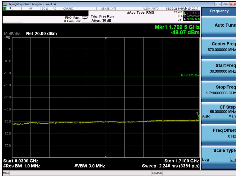
Plot 7-78. Conducted Spurious Plot (Band 4 – 15.0MHz QPSK – RB Size 1, RB Offset 0 – High Channel)
