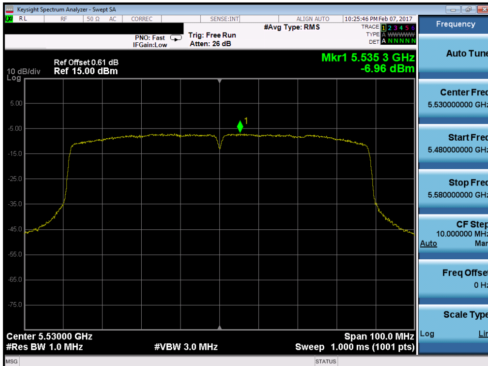
Plot 7-106. Power Spectral Density Plot (80MHz BW 802.11ac (UNII Band 2C) – Ch. 106)
