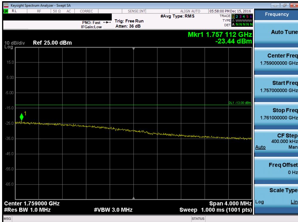
Plot 7-96. Upper Extended Band Edge Plot (Band 4 – 5.0MHz QPSK – RB Size 25)
