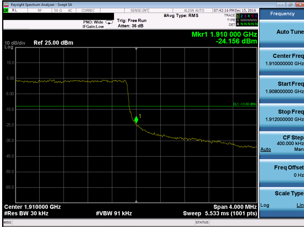
Plot 7-115. Upper Band Edge Plot (Band 2 – 3.0MHz QPSK – RB Size 15)
