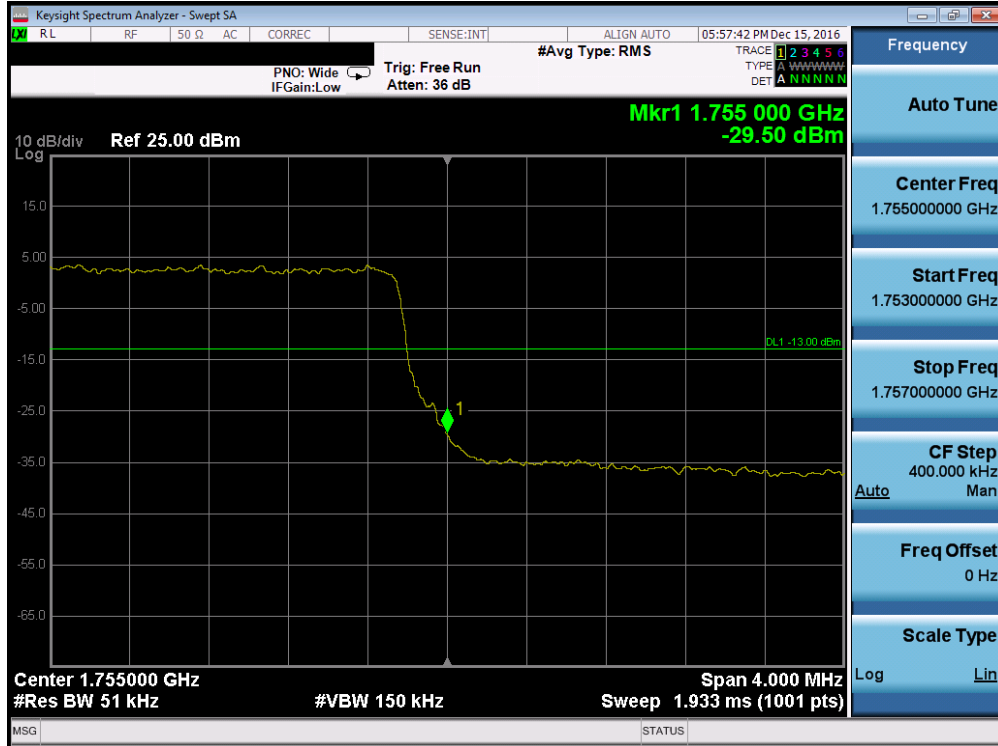
Plot 7-95. Upper Band Edge Plot (Band 4 – 5.0MHz QPSK – RB Size 25)
