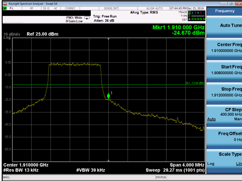
Plot 7-111. Upper Band Edge Plot (Band 2 – 1.4MHz QPSK – RB Size 6)
