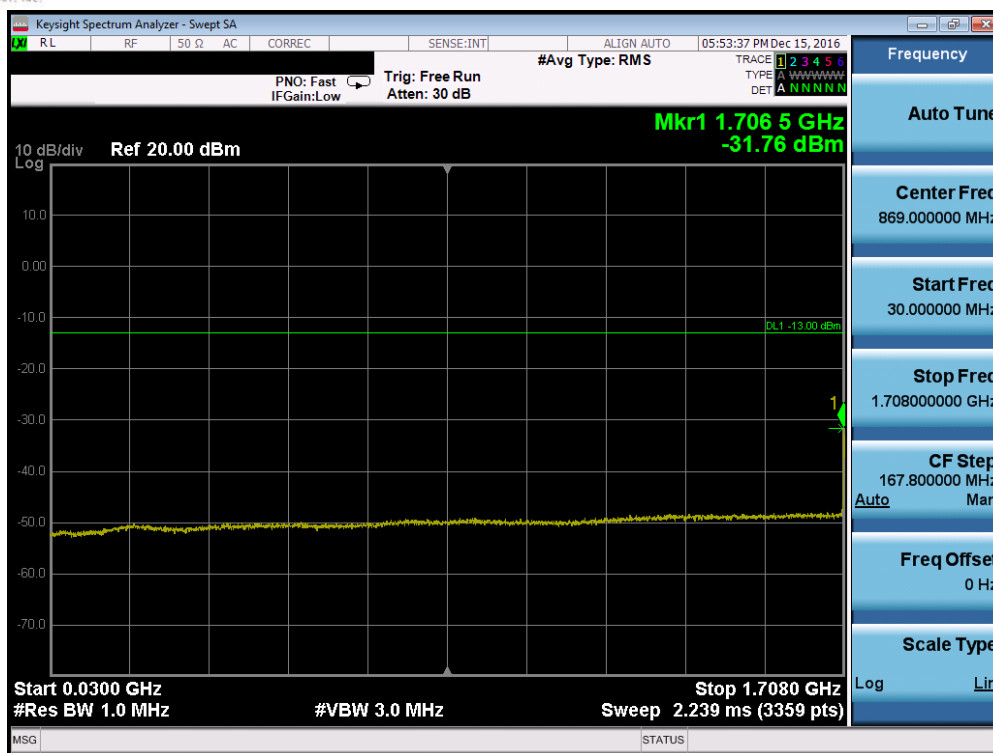
Plot 7-55. Conducted Spurious Plot (Band 4 – 5.0MHz QPSK – RB Size 1, RB Offset 0 – Low Channel)
