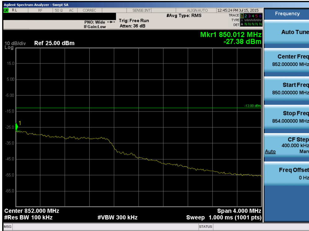
Plot 6-117. Upper Extended Band Edge Plot (Band 5/26 – Band 5 – 3.0MHz QPSK – RB Size 15)
