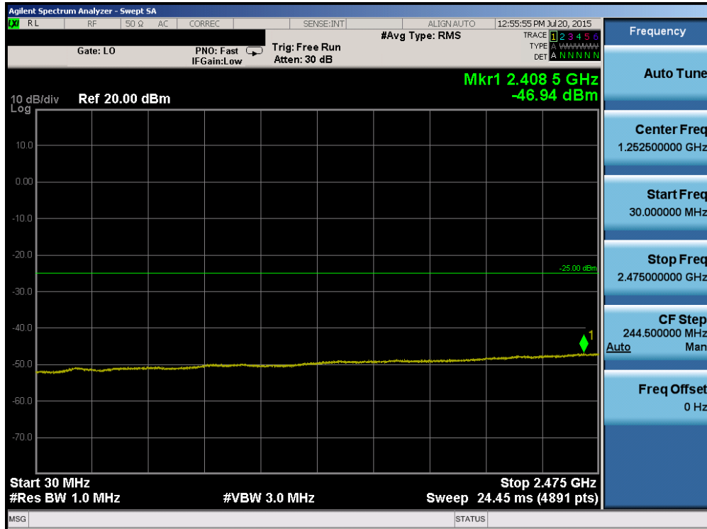
Plot 6-87. Conducted Spurious Plot (Band 41 – 10.0MHz QPSK – RB Size 1, RB Offset 0– Low Channel)
