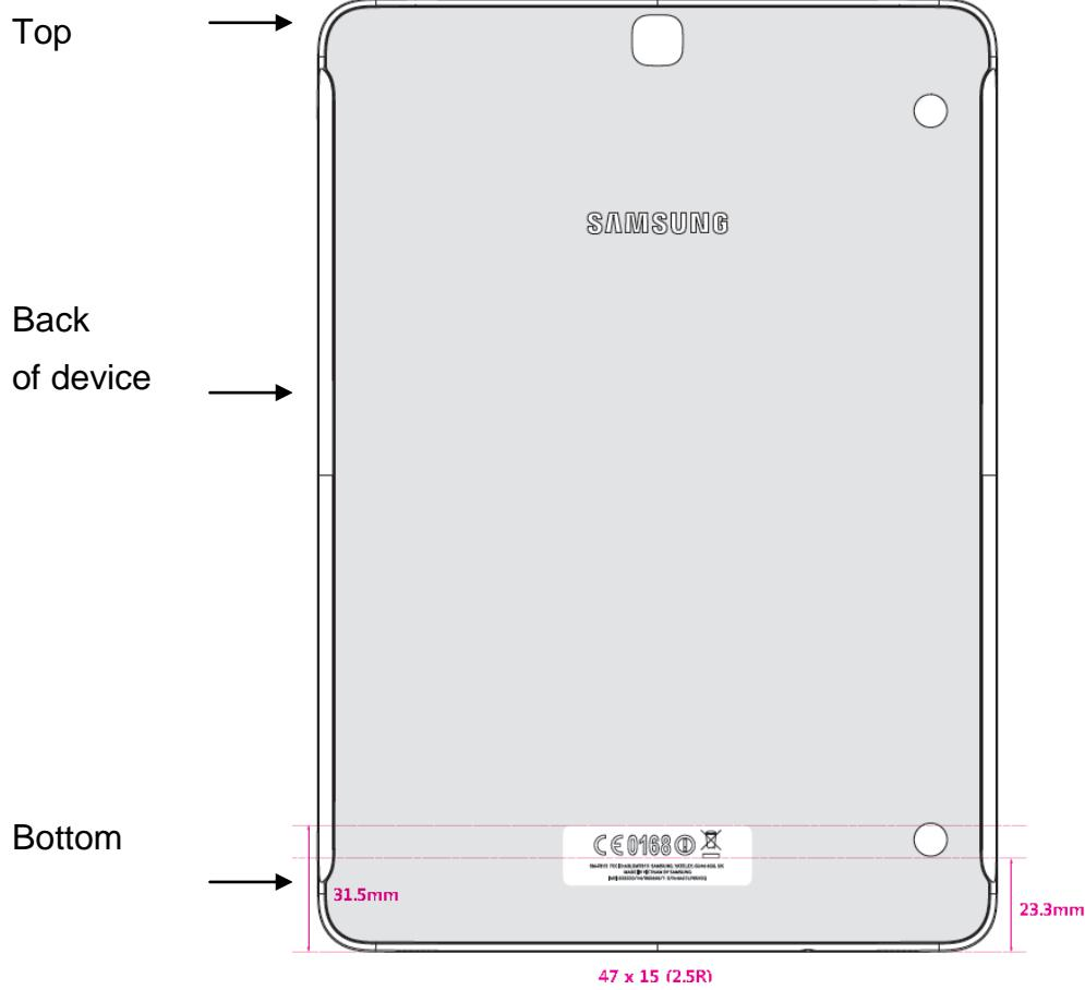
Tablet : FCC ID is engraved on bottom of the device
