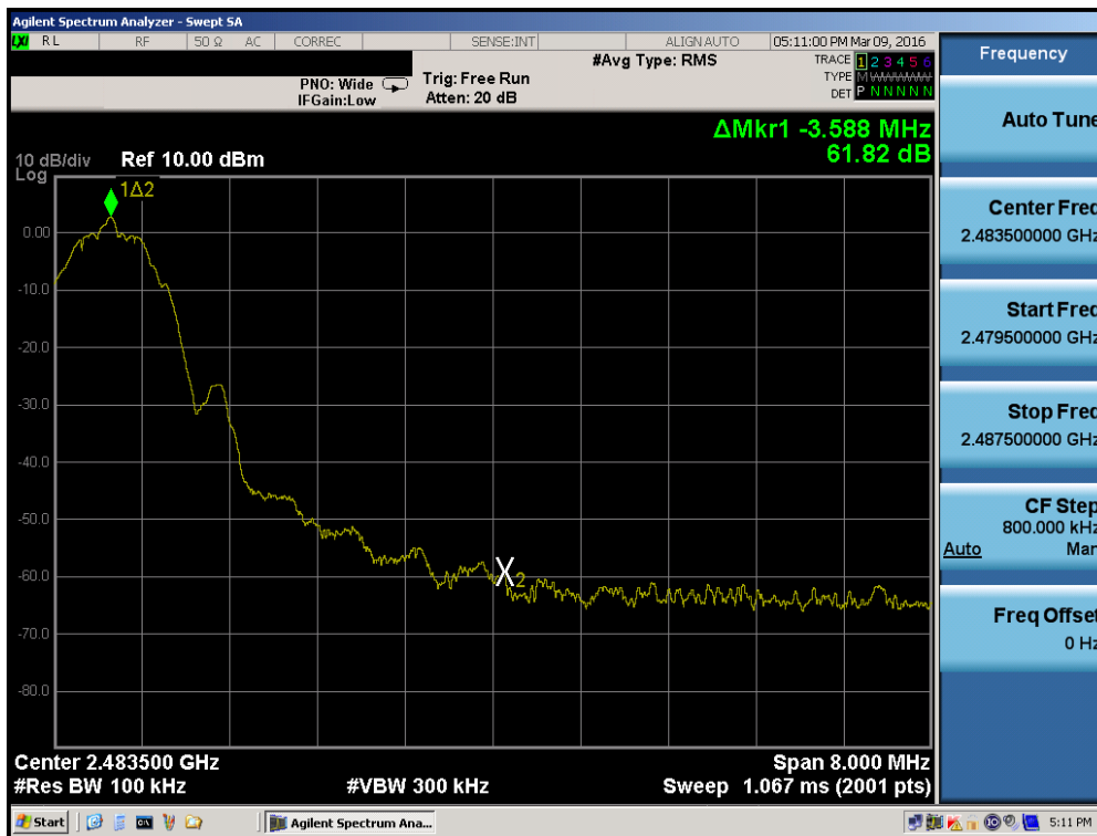
Plot 7-11. Band Edge Plot (Bluetooth (LE) – Ch. 39)
