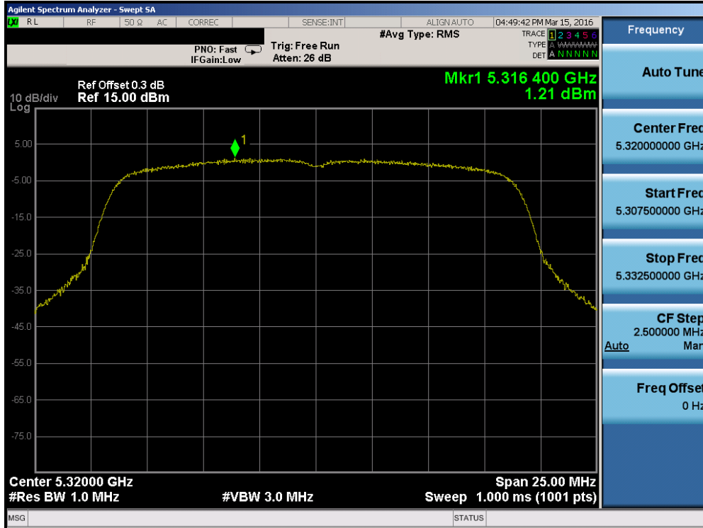
Plot 7-93. Power Spectral Density Plot (20MHz BW 802.11n (UNII Band 2A) – Ch. 64)
