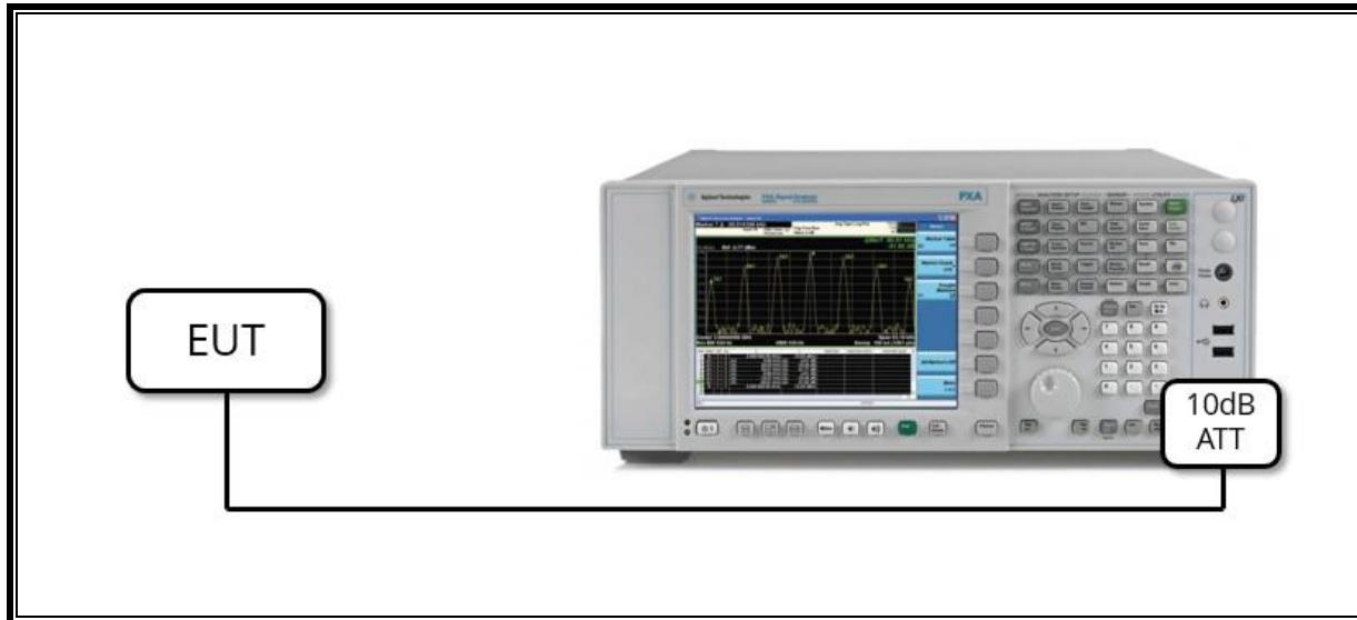
**SETUP DIAGRAM FOR TESTS (RADIATED TEST SETUP)**
