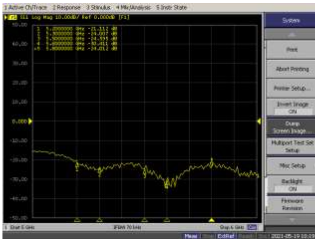
< Figure 1. Measurement result of Head Return Loss >
