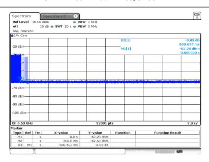
Channel move time = 0.800 625 sClosing time =  $0.000 625 \text{ s} \times 12 = 0.007 500 \text{ s}$
