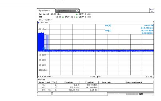
Channel move time = 0.818750 sClosing time =  $0.000625 \text{ s} \times 13 = 0.008125 \text{ s}$
