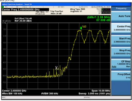
Test Plots with hopping (GFSK)
