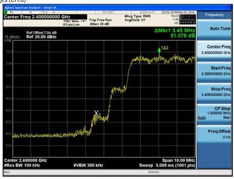
Test Plots with hopping ( $\pi/4DQPSK$ )
