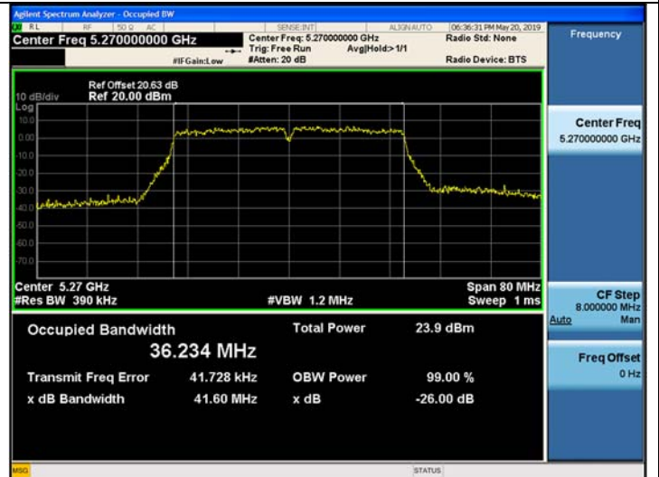
802.11n_HT40 UNII 3 BAND 26dB Bandwidth (CH 151)
