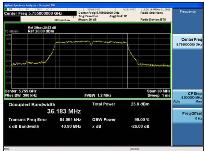
802.11ac_VHT40 UNII 3 BAND 26dB Bandwidth (CH 151)
