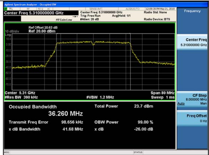
802.11ac_VHT40 UNII 3 BAND 26dB Bandwidth (CH 151)
