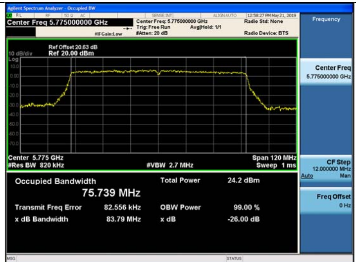
802.11ac_VHT80 UNII 3 BAND 26dB Bandwidth (CH 155)
