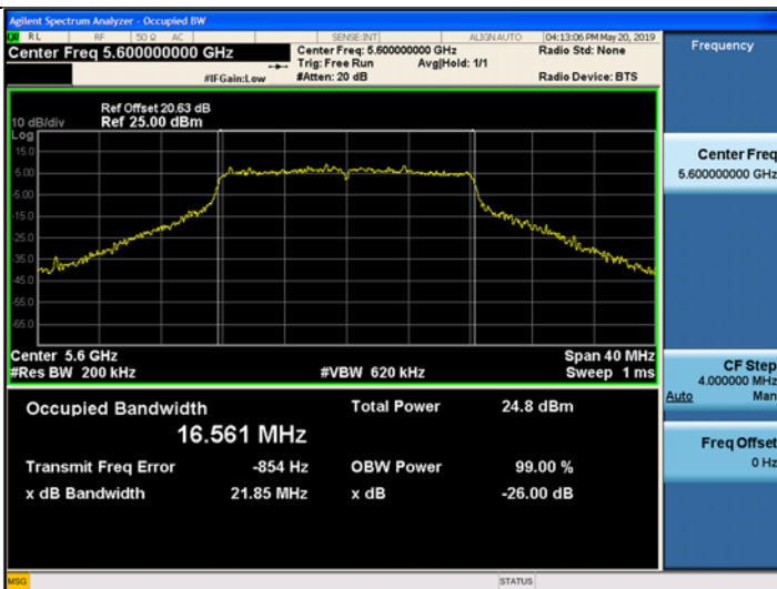
802.11a UNII 2C BAND 26dB Bandwidth (CH120)
