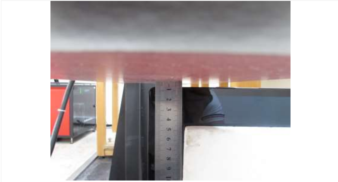
Distance of 6 mm from the EUT
