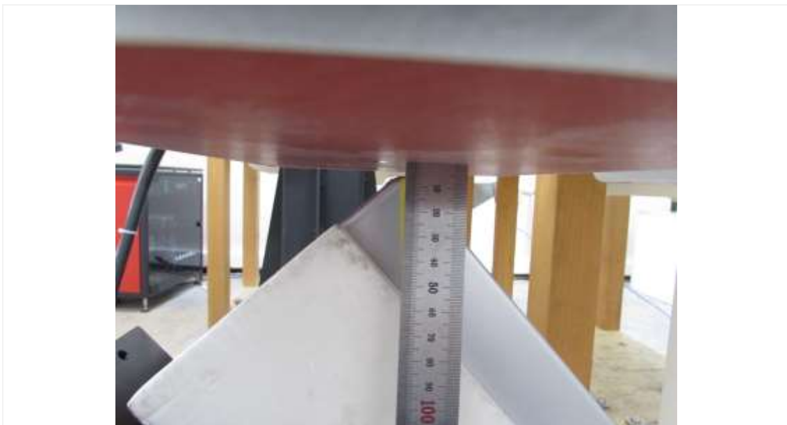
Distance of 6 mm from the EUT
