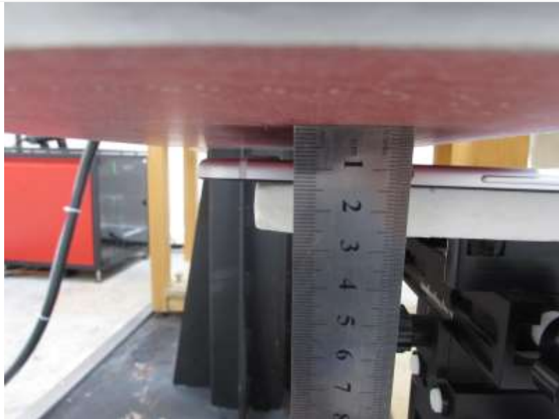
Distance of 8 mm from the EUT
