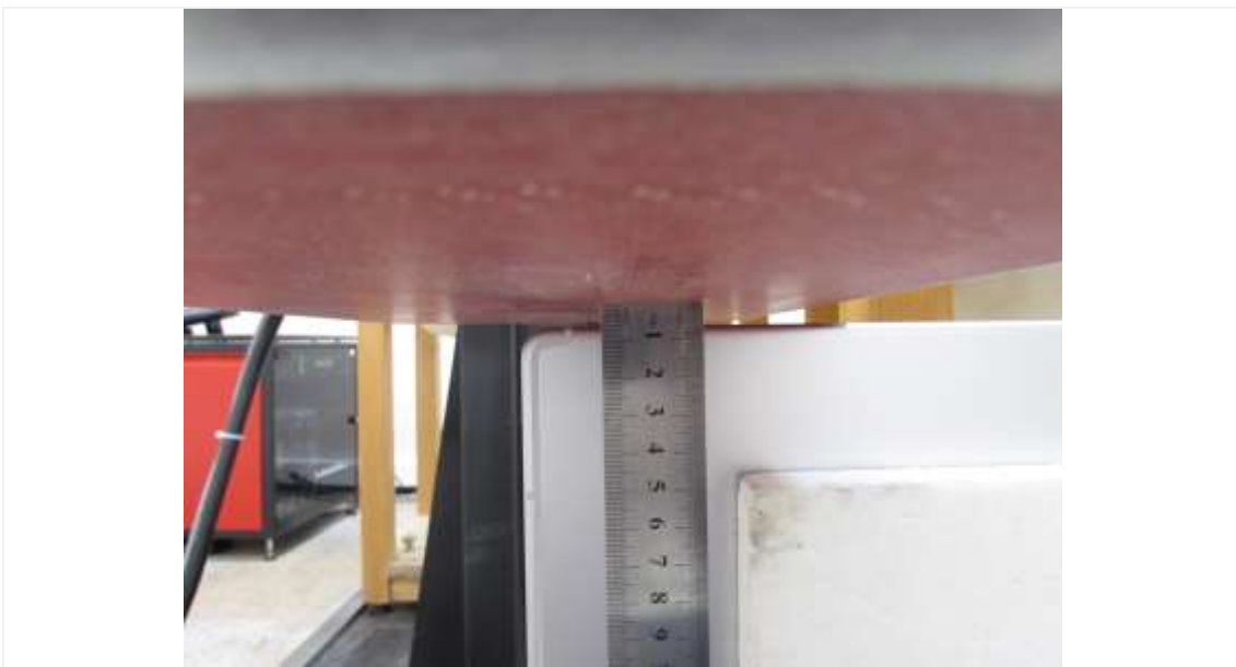
Distance of 6 mm from the EUT
