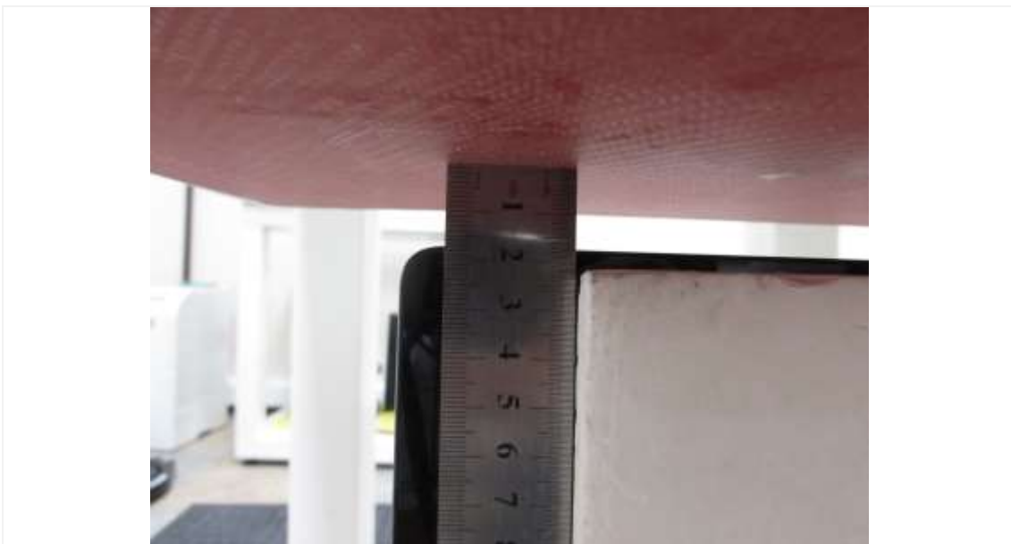
Distance of 17 mm from the EUT
