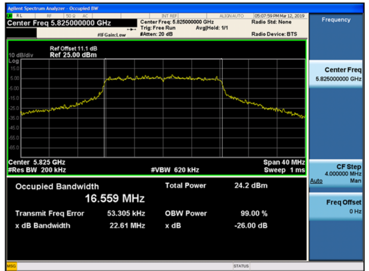
802.11a UNII 3 BAND 26dB Bandwidth (CH 165)
