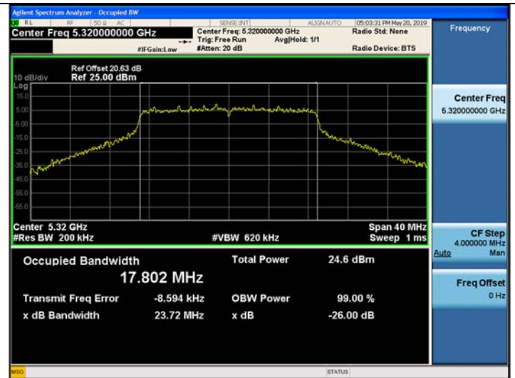
802.11n_HT20 UNII 3 BAND 26dB Bandwidth(CH 165)
