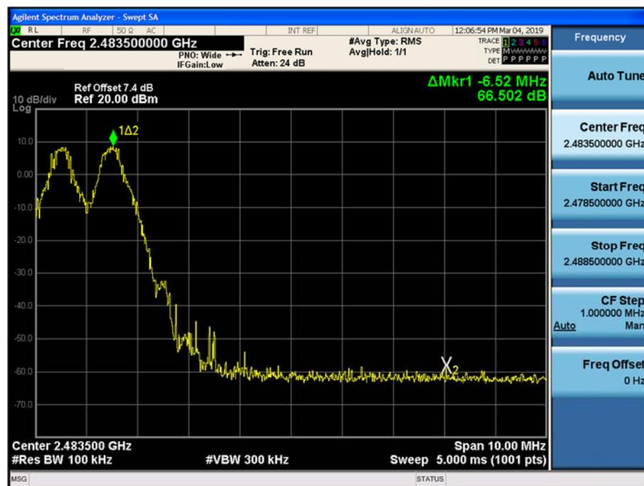
Test Plots with hopping (8DPSK)
