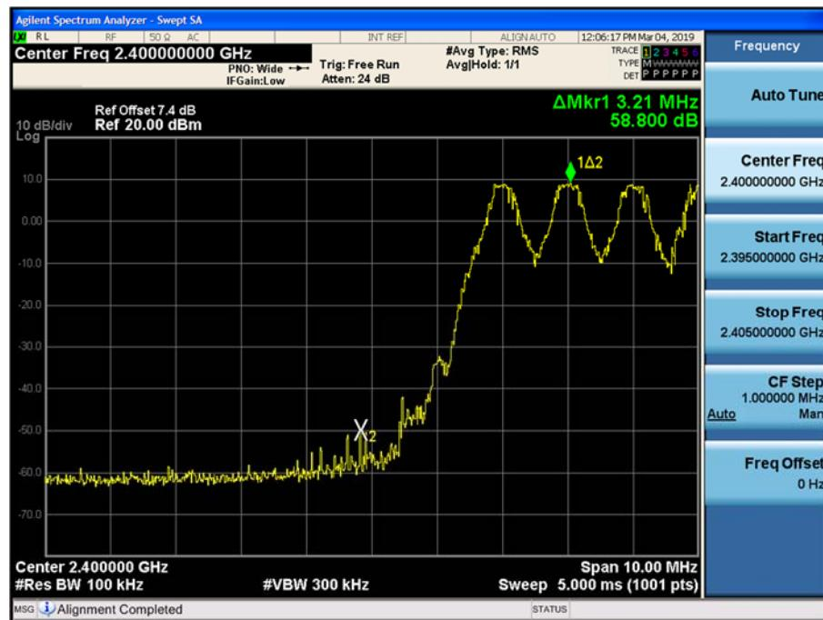
Test Plots with hopping (GFSK)
