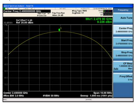
Test Plots (8DPSK) Peak Power (CH.0)
