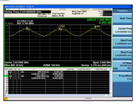
Test Plots (8DPSK) Channel Separation
