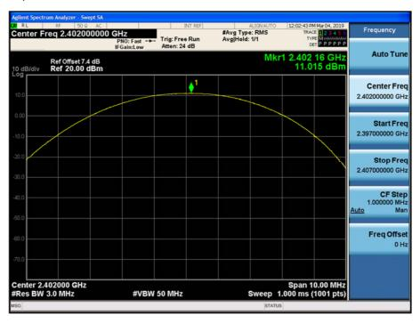
Test Plots (π/4DQPSK) Peak Power (CH.39)
