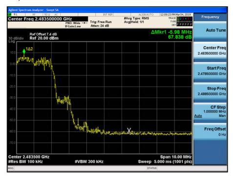
Test Plots with hopping ( $\pi$ /4DQPSK) Band Edges (CH.0)
