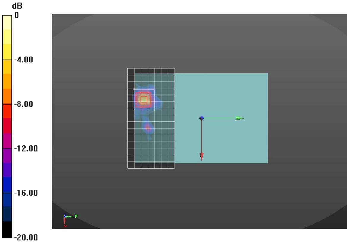
According to KDB 248227 D01v02r02 section 6.1: "When antennas are spatially separated to the extent that SAR distributions do not overlap and can be treated independently, SAR compliance for simultaneous transmission is determined separately for each individual antenna".
