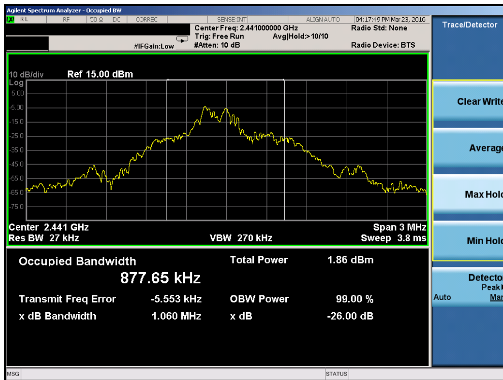
Plot 7-1. Occupied Bandwidth Plot (ANT+ – Ch. 39)
