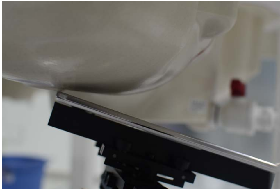
SAR Test Setup Photo 2 – Right Tilt
