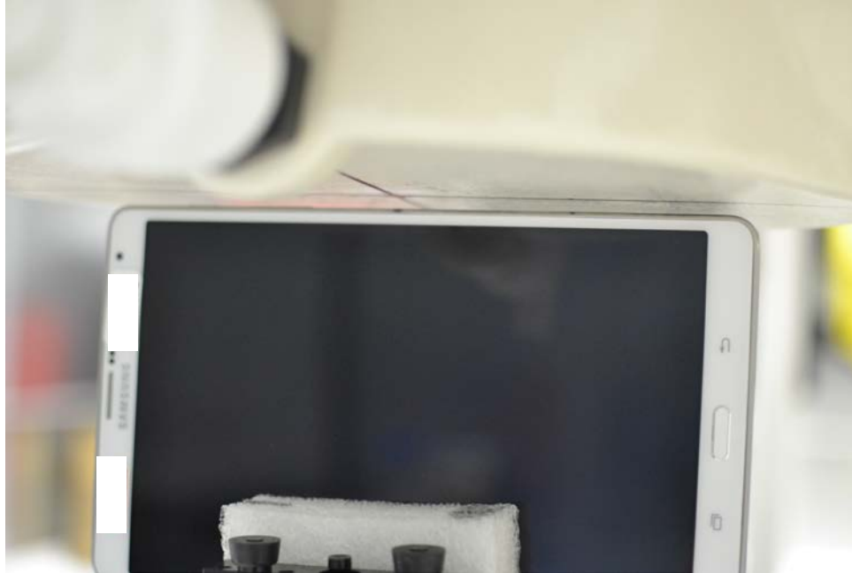
SAR Test Setup Photo 11 – Right Edge at 4 mm
