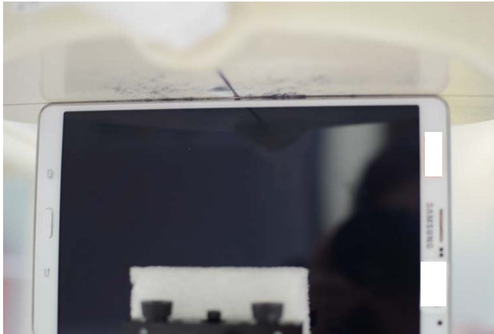
SAR Test Setup Photo 12 – Left Edge at 0.0 mm
