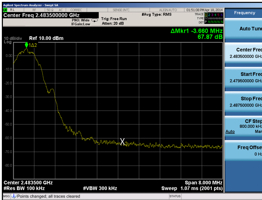
Plot 6-11. Band Edge Plot (Bluetooth (LE) – Ch. 39)
