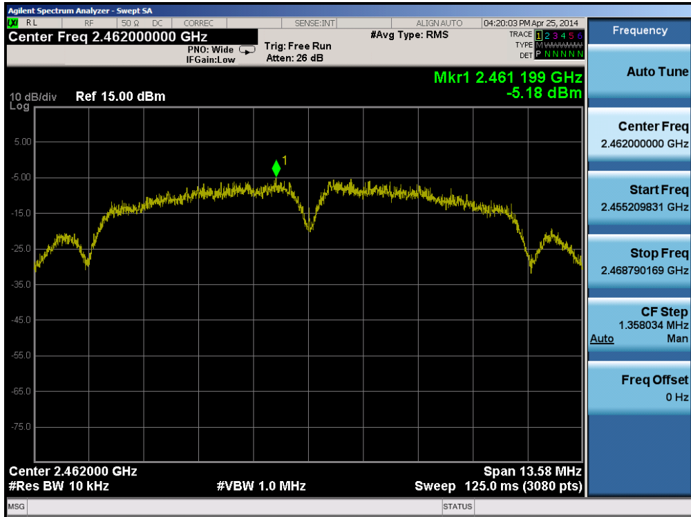
Plot 6-39. Power Spectral Density Plot (802.11b – Ch. 11)
