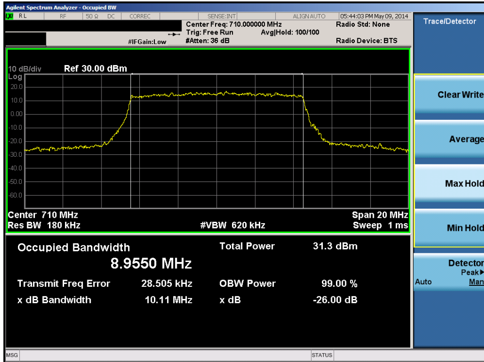
Plot 6-3. Occupied Bandwidth Plot (Band 17 – 10.0MHz QPSK – RB Size 50)
