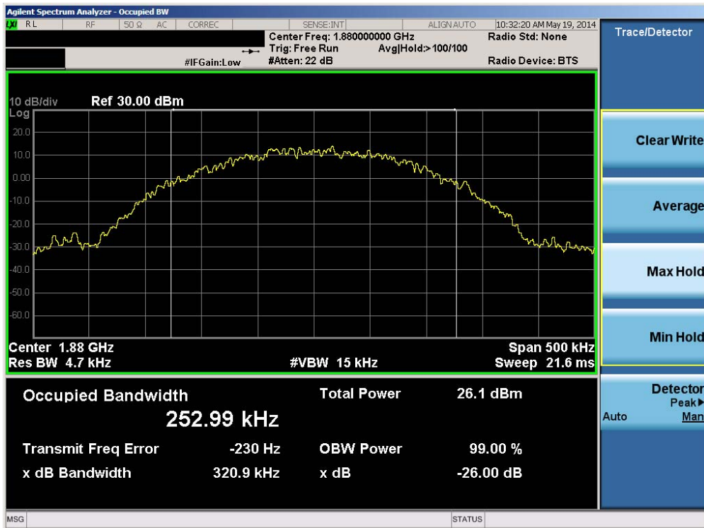
Plot 6-4. Occupied Bandwidth Plot (EDGE1900 Mode – Ch. 661)
