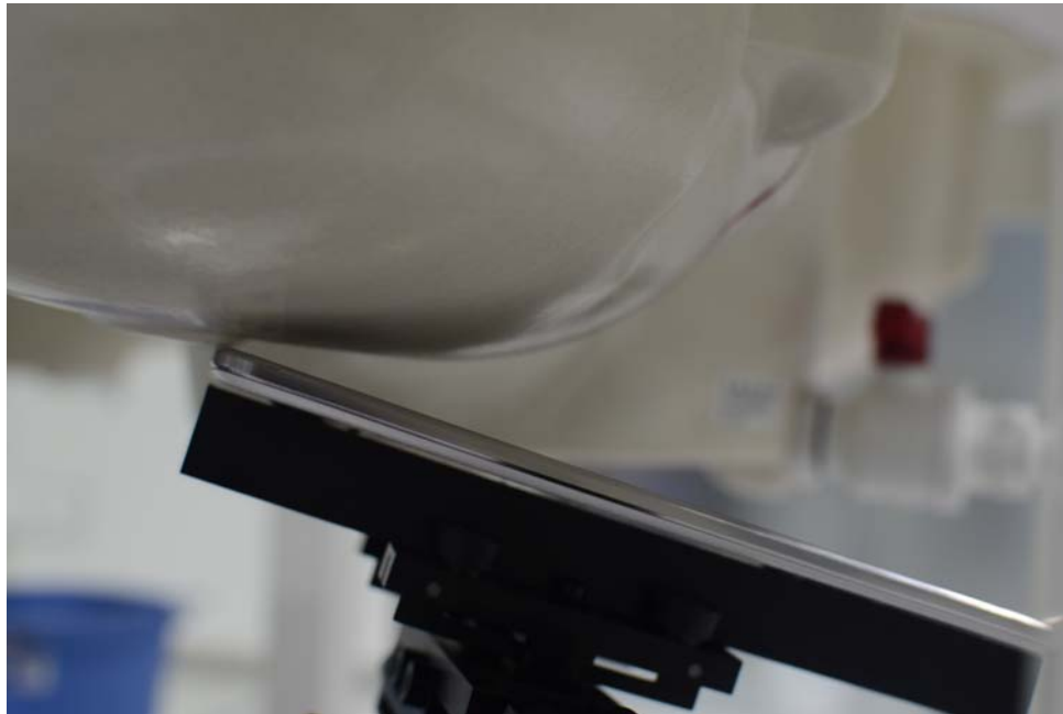
SAR Test Setup Photo 2 – Right Tilt
