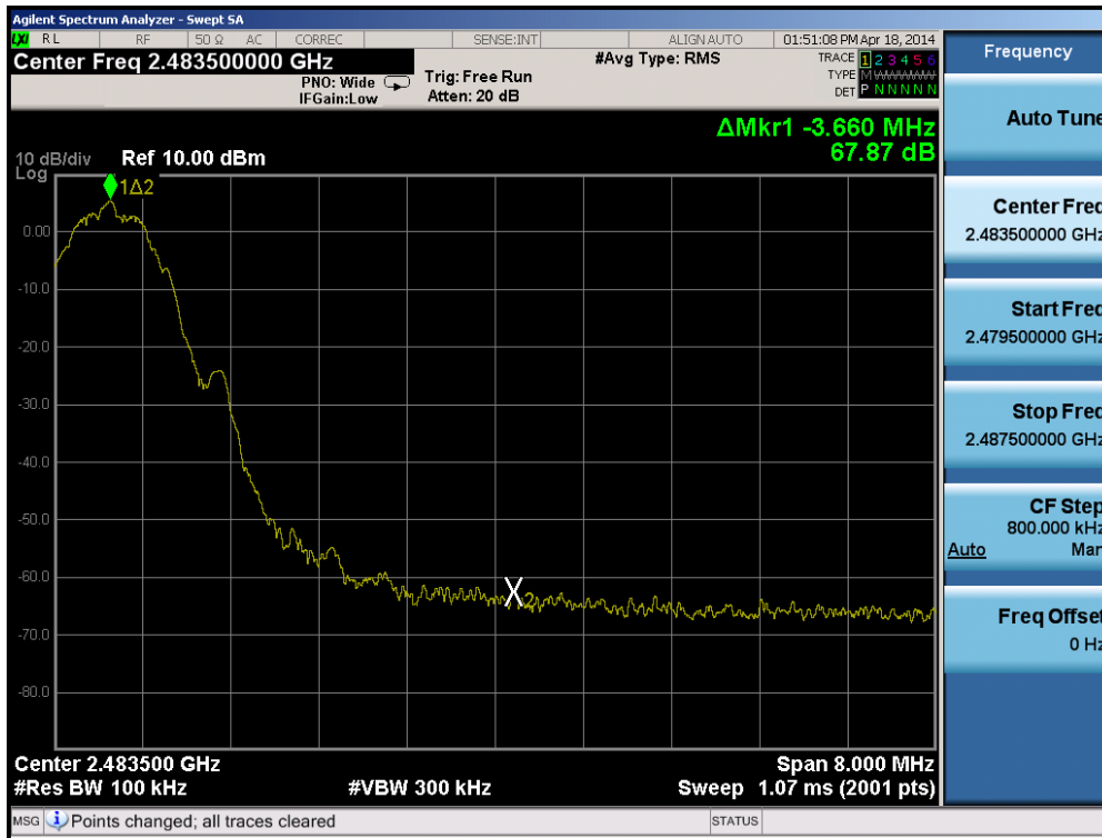
Plot 6-11. Band Edge Plot (Bluetooth (LE) – Ch. 39)
