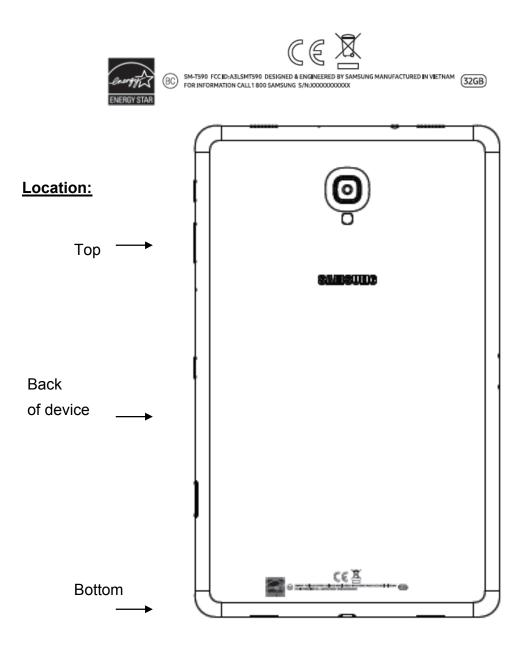
Tablet: FCC ID is engraved on rear bottom of the device.
