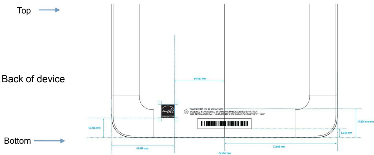
FCC ID is engraved on rear bottom of the device.
