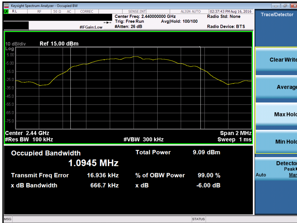
Plot 7-2. 6dB Bandwidth Plot (Bluetooth (LE) – Ch. 19)
