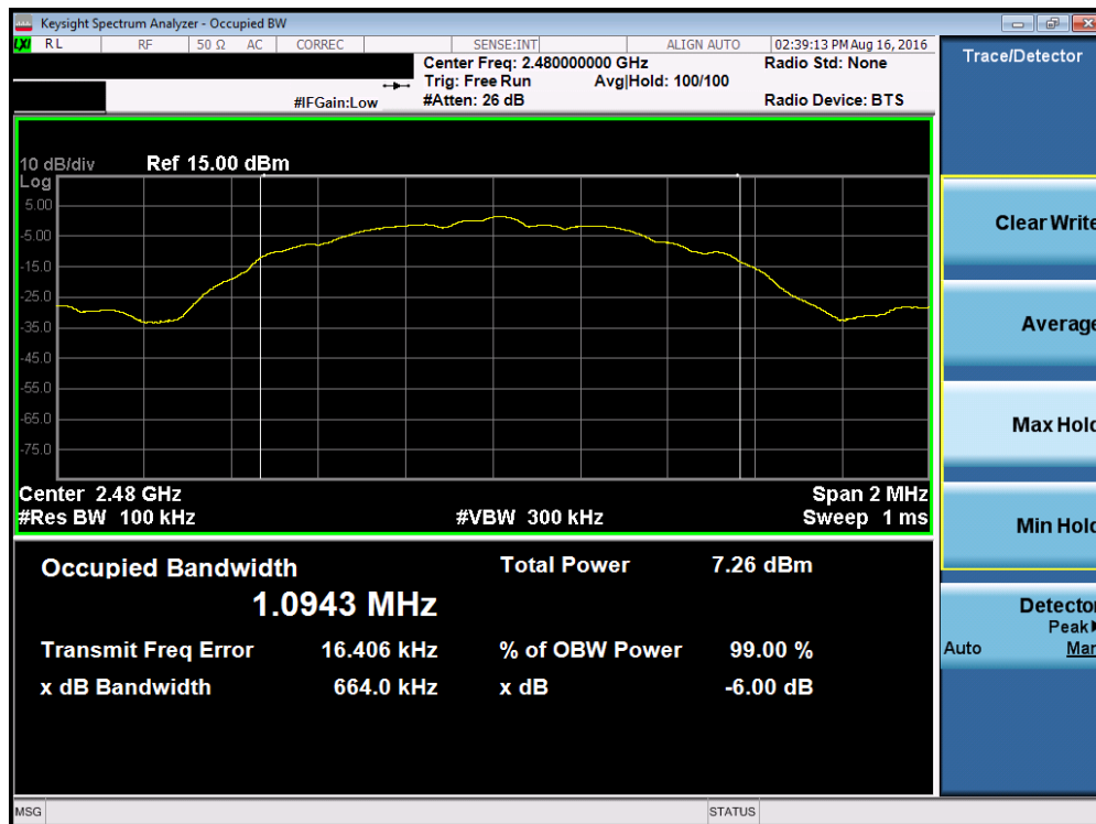
Plot 7-3. 6dB Bandwidth Plot (Bluetooth (LE) – Ch. 39)
