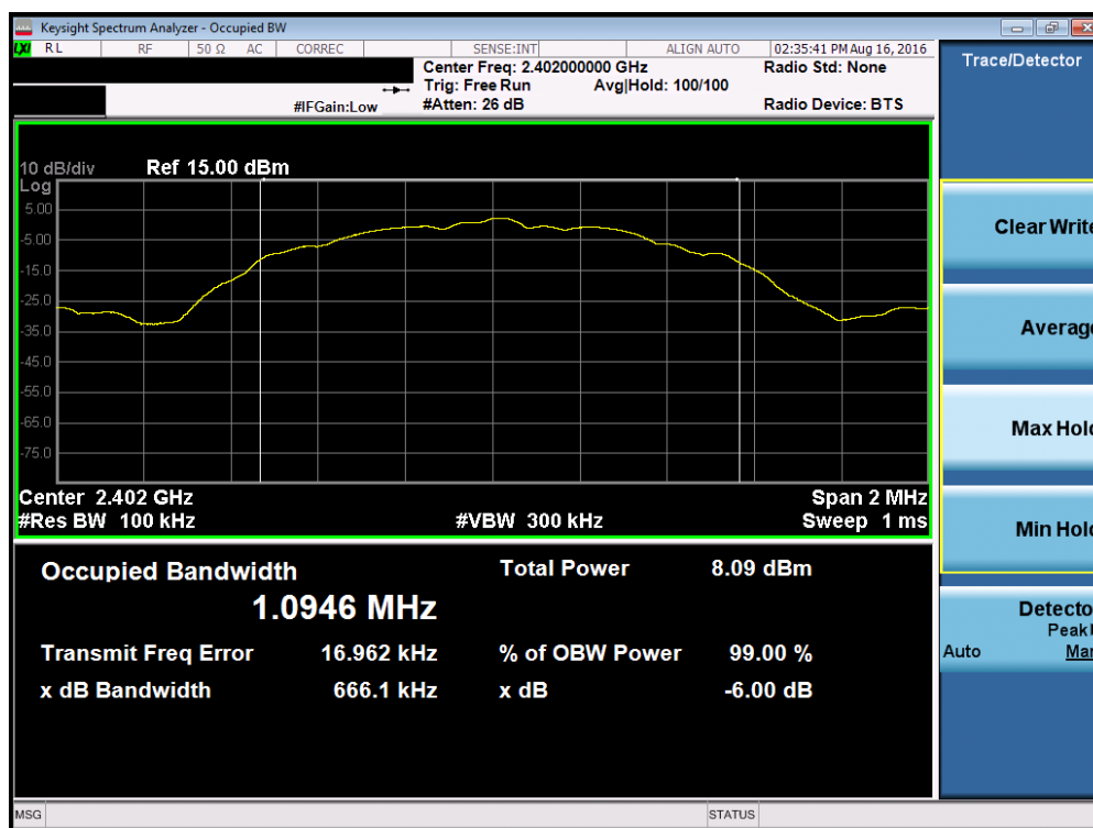
Plot 7-1. 6dB Bandwidth Plot (Bluetooth (LE) – Ch. 0)
