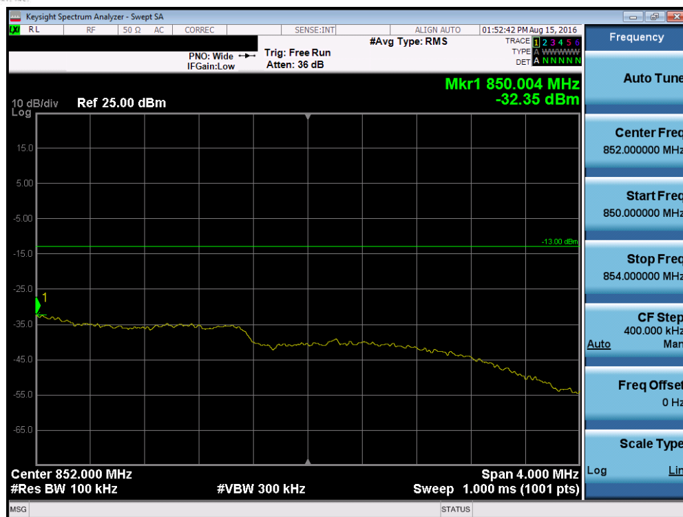
Plot 7-65. Upper Extended Band Edge Plot (Band 26 – Band 5 – 3.0MHz QPSK – RB Size 15)
