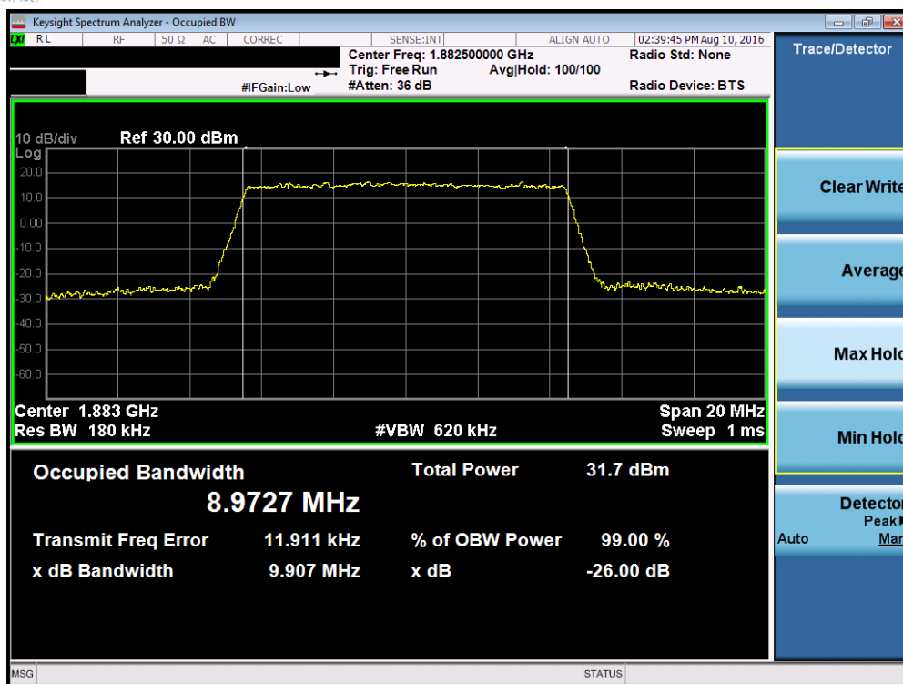
Plot 7-17. Occupied Bandwidth Plot (Band 25 – 10.0MHz QPSK – RB Size 50)
