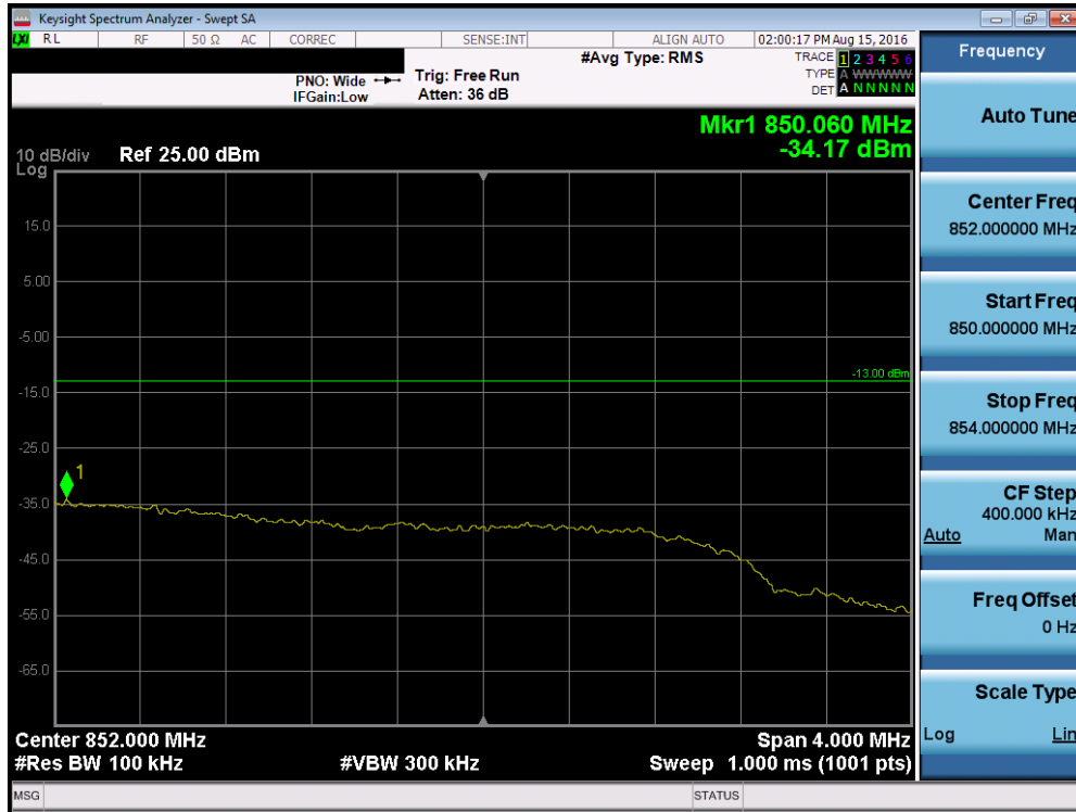
Plot 7-69. Upper Extended Band Edge Plot (Band 26 – 5.0MHz QPSK – RB Size 25)
