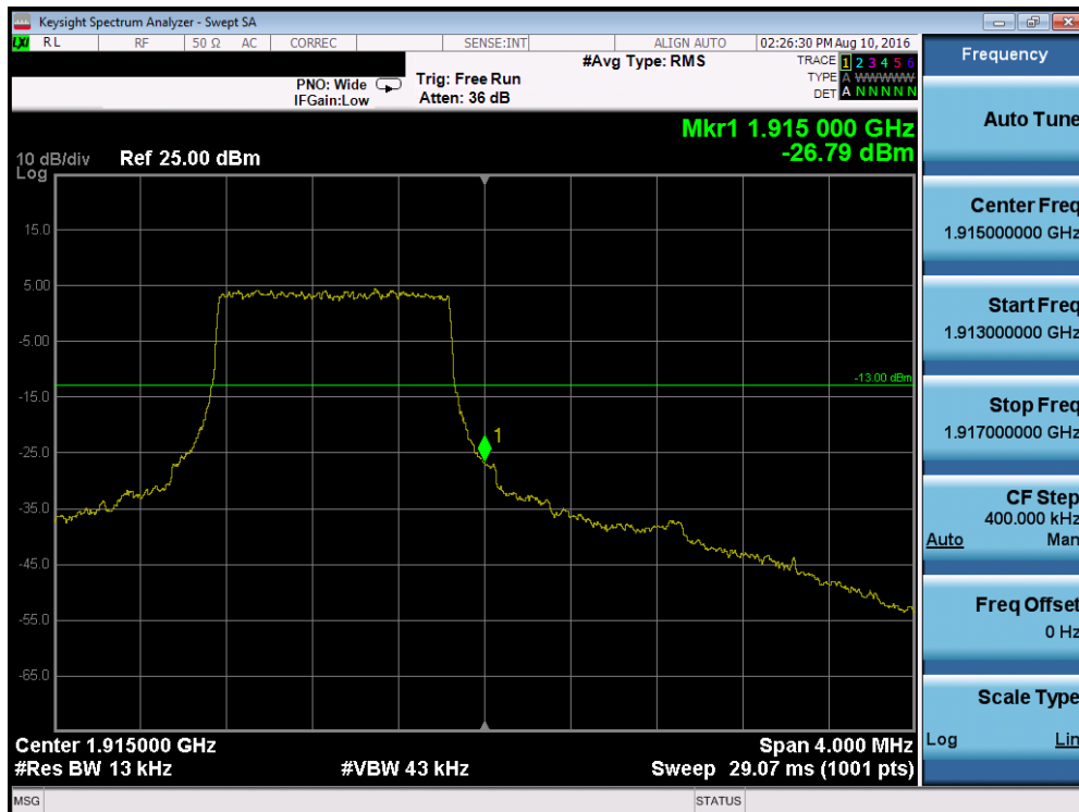
Plot 7-76. Upper Band Edge Plot (Band 25 – 1.4MHz QPSK – RB Size 6)
