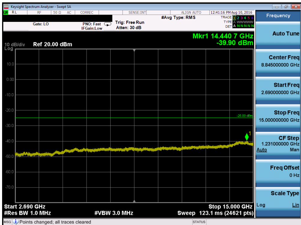
Plot 7-56. Conducted Spurious Plot (Band 41 – 5.0MHz QPSK – RB Size 1, RB Offset 0 – High Channel)
