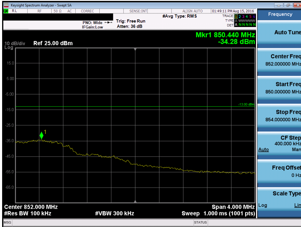
Plot 7-61. Upper Extended Band Edge Plot (Band 26 – 1.4MHz QPSK – RB Size 6)
