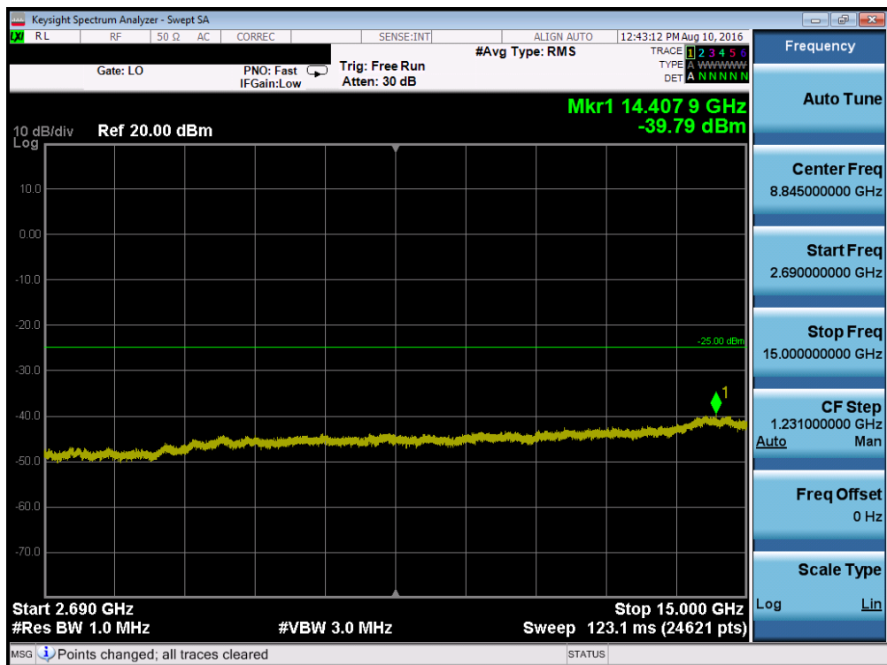
Plot 7-50. Conducted Spurious Plot (Band 41 – 5.0MHz QPSK – RB Size 1, RB Offset 0 – Low Channel)
