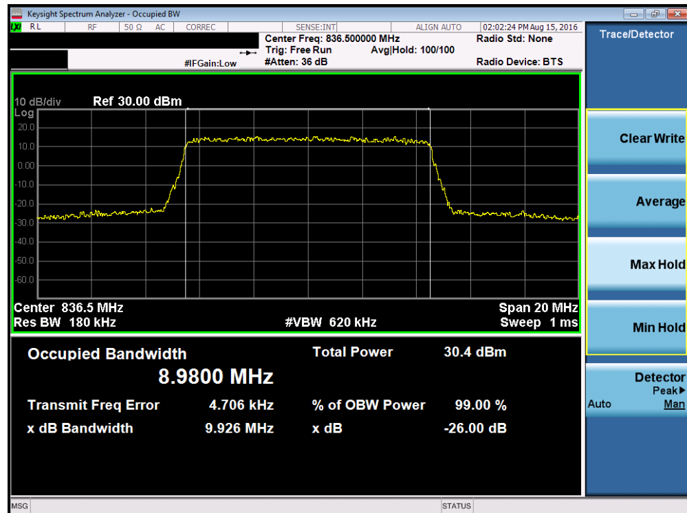
Plot 7-8. Occupied Bandwidth Plot (Band 26 – 10.0MHz 16-QAM – RB Size 50)
