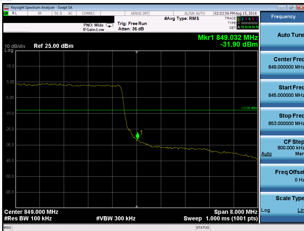
Plot 7-71. Upper Band Edge Plot (Band 26 – 10.0MHz QPSK – RB Size 50)
