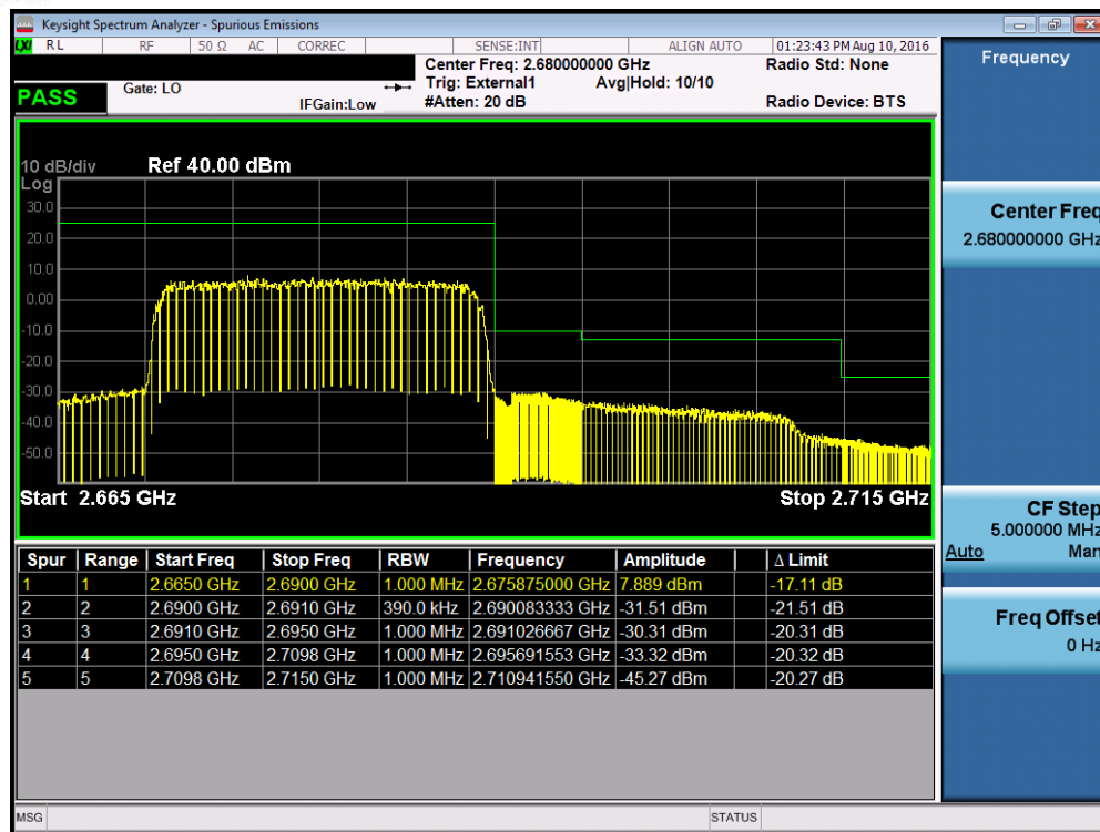
Plot 7-105. Upper ACP Plot (Band 41 – 20.0MHz QPSK – RB Size 100)
