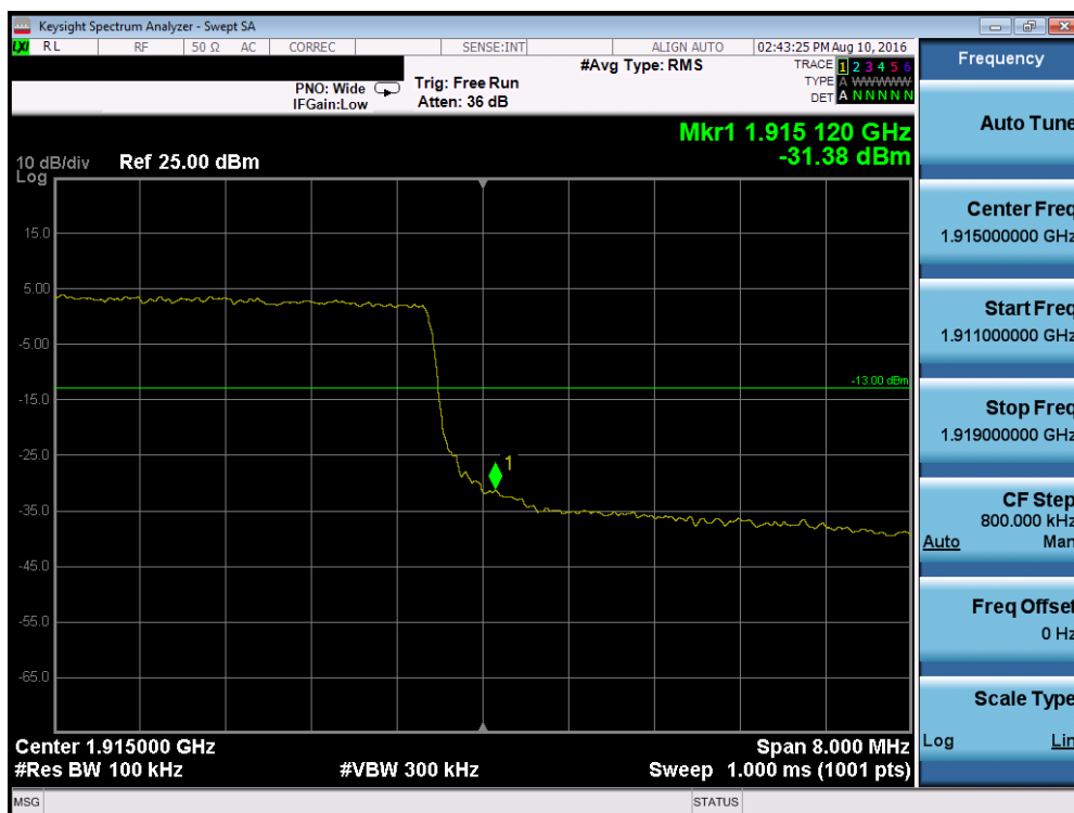
Plot 7-88. Upper Band Edge Plot (Band 25 – 10.0MHz QPSK – RB Size 50)
