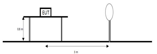
The diagram below shows the test setup that is utilized to make the measurements for emission from 30 Mb to 1 GHz emissions.
