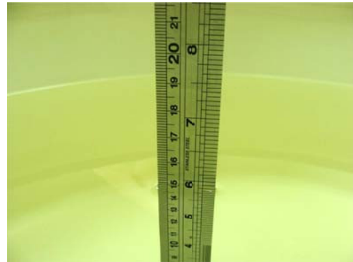
Photo of Liquid Height for Body SAR
