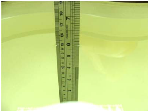
Photo of Liquid Height for Head SAR
