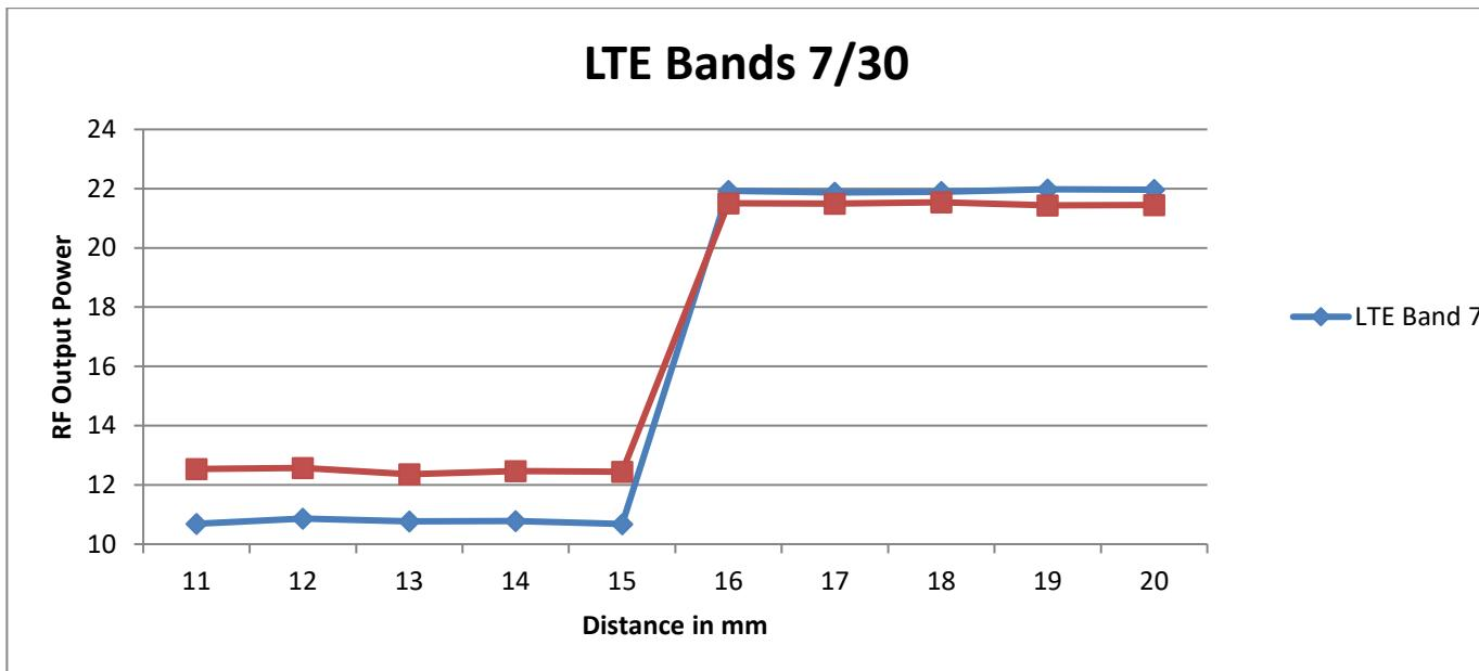
Edge 1, DUT Moving Toward (Trigger) and Away (Release) from the Phantom
