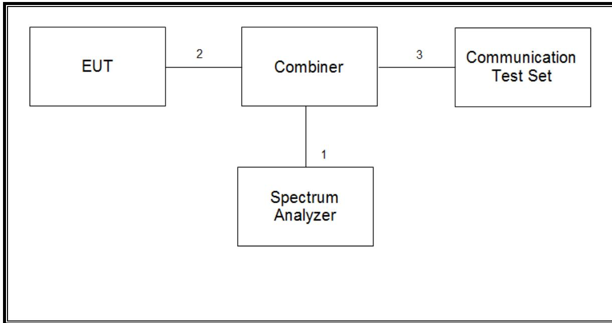
**SETUP DIAGRAM FOR TESTS (RADIATED TEST SETUP)**
